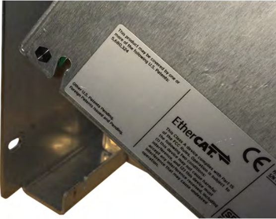
Figure 2 Notch for Module Alignment
