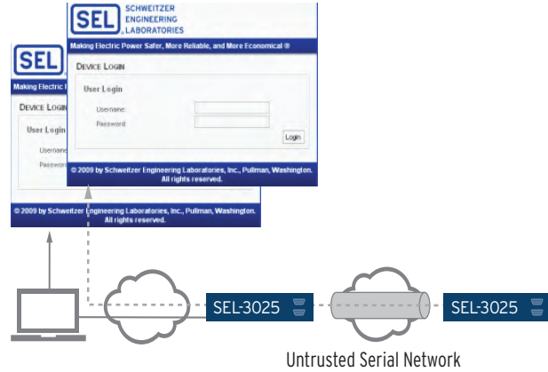
----- Authenticated/Encrypted Communication Figure 5 Nonintrusive HTTPS and Remote Management Client
