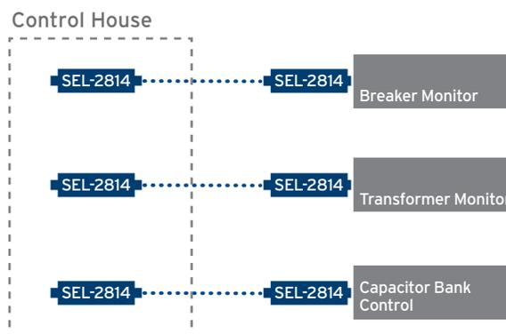
Transfer information between remote equipment and the control house in even the largest stations.
