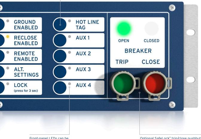
Front-panel LEDs can be programmed to indicate custom alarms.
