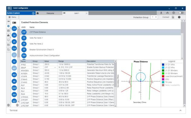
Grid Configurator's visualization tools help you easily adjust a device's protection elements.
