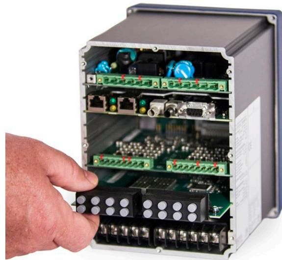
Order either four or eight arc-flash sensor inputs.
