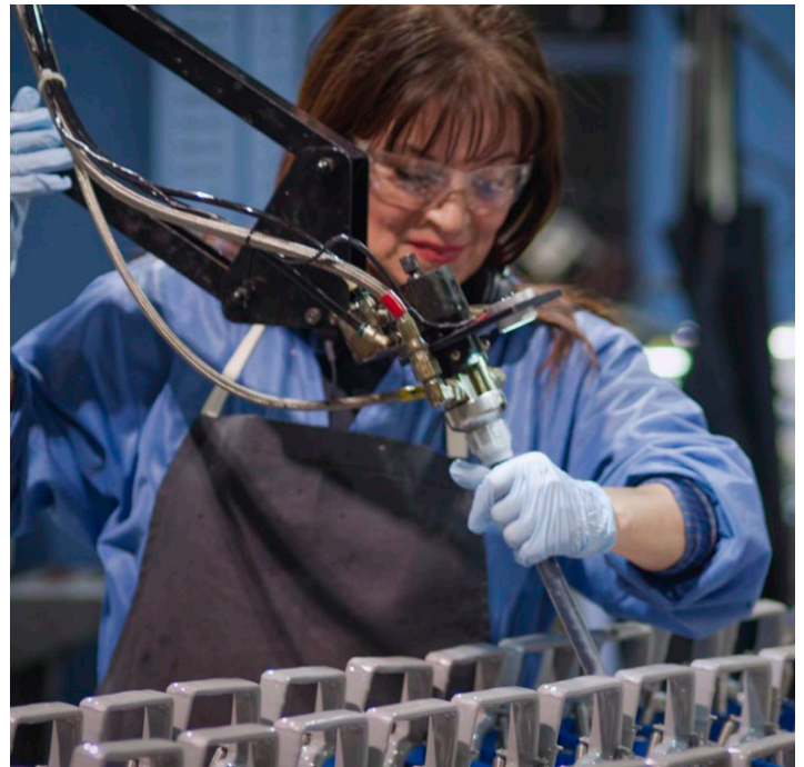
An SEL employee is applying a potting compound to seal the SEL-SCT metal laminations for water resistance.
