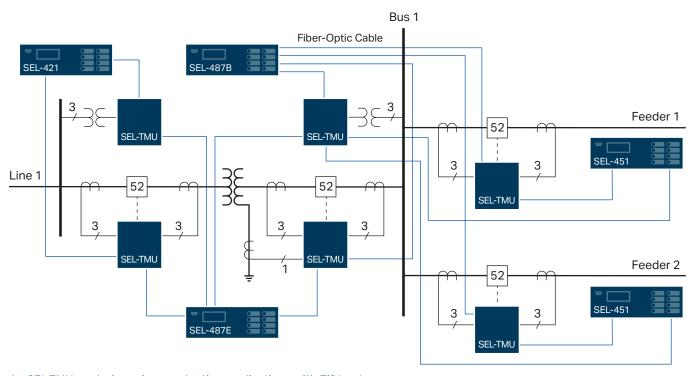
An SEL-TMU works in various protection applications with TiDL relays.
