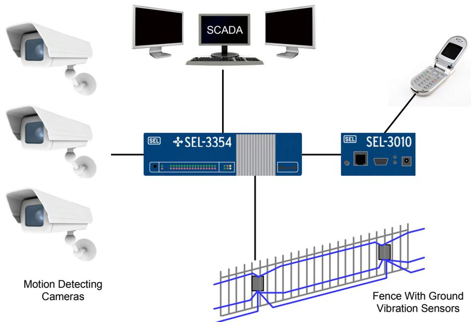
Figure 1 Physical Surveillance System
