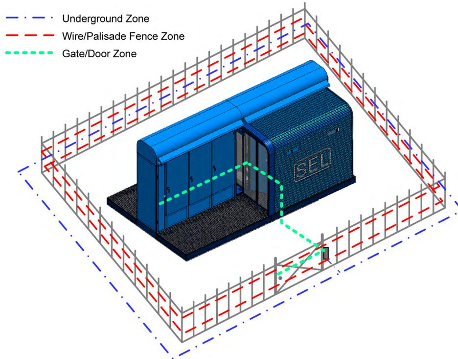
Figure 2 Typical Perimeter Security Monitoring
