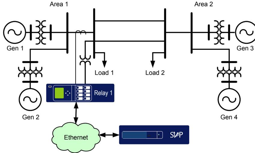
Figure 1 Power System Model Using Modal Analysis to Monitor Inter-Area Oscillation
