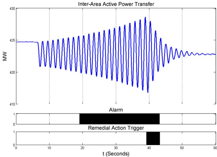
Figure 2 Inter-Area Power Oscillation and Modal Analysis System Outputs
