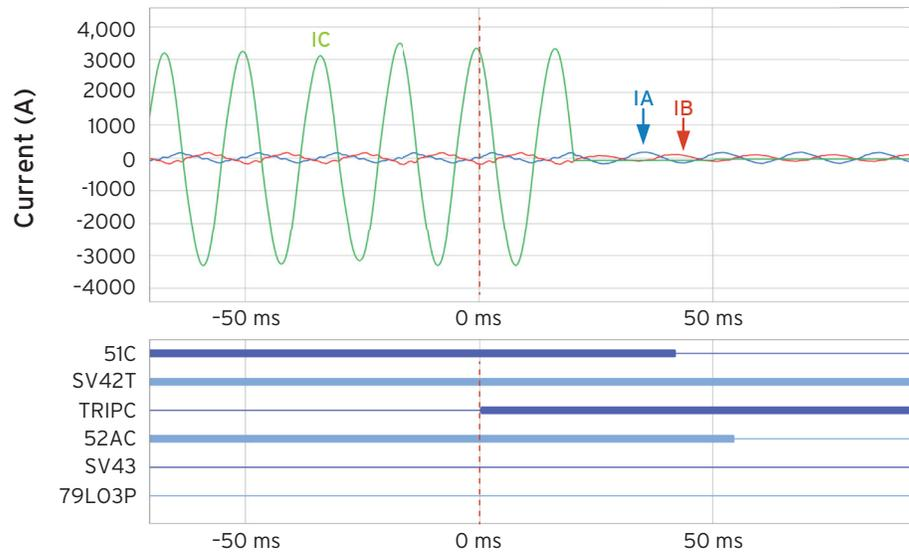
Figure 12—The first trip event for the fault.
