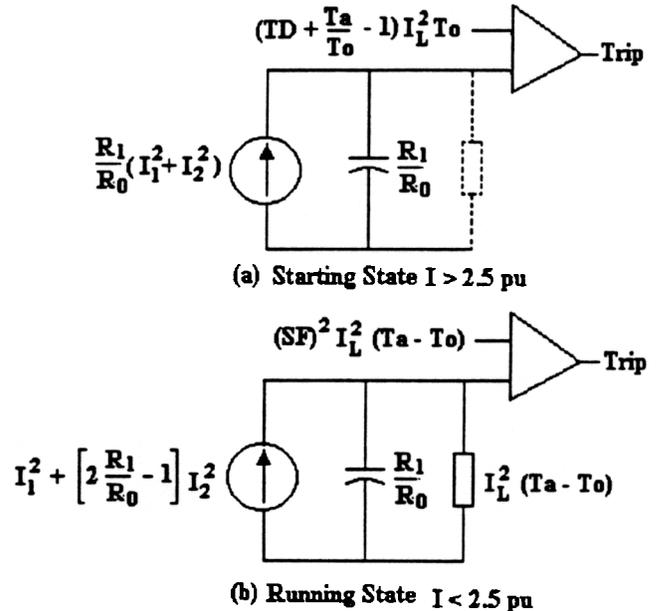
Figure 5: States of the Thermal Model
