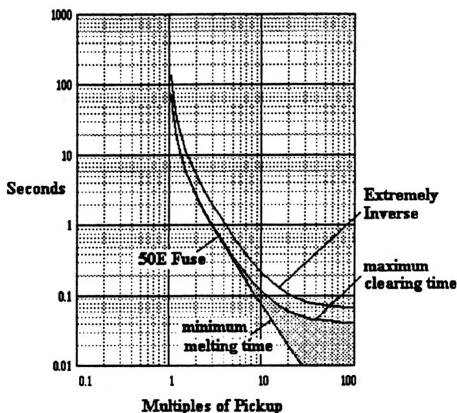
Figure 2: Extremely Inverse Characteristic Compared with Min. Melting and Maximum Clearing Time of a 50E Fuse
