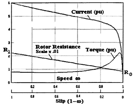
Figure 4: Current, Torque, and Rotor Resistance of an Induction Motor Versus Speed
