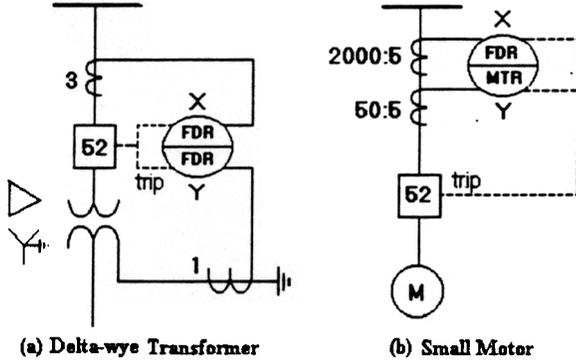
Figure 6: Applications of a Dual Universal Overcurrent Relay
