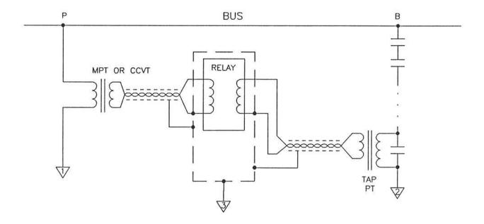
Figure 14: Ground References for Capacitor Protection
