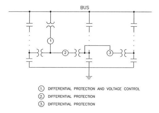
Figure 13: Fuseless Shunt Capacitor Bank Protection
