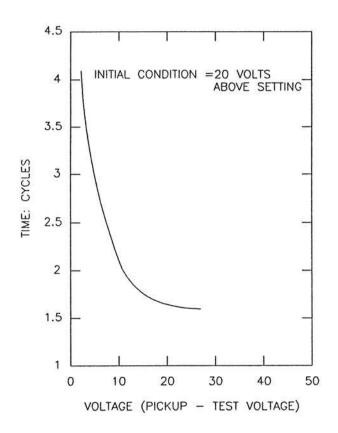
Figure 11: Undervoltage Element Dynamic Response
