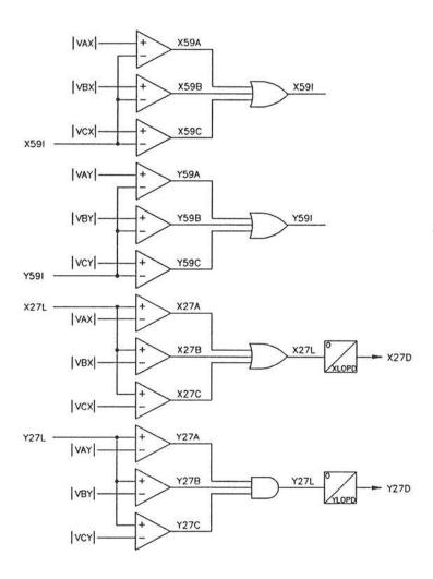
Figure 4: Overvoltage Elements / Undervoltage Elements and Logic
