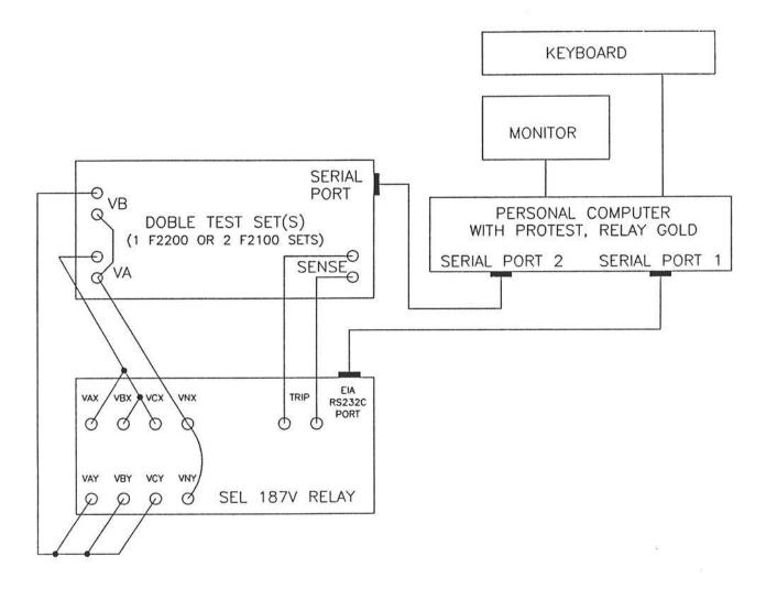
Figure 9: Block Diagram for Automated Tests
