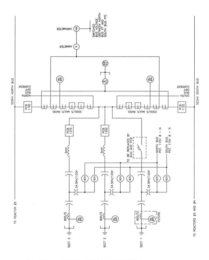
Figure 17: Raver Capacitor Bank Control and Protection
