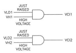
Figure 8: Voltage Control Instability Logic
