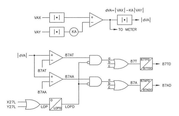
Figure 6: Voltage Differential Protection (Per Phase)
