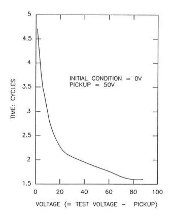
Figure 10: Overvoltage Element Dynamic Response
