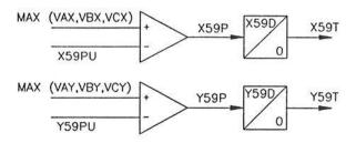
Figure 5: Definite-Time Overvoltage Logic
