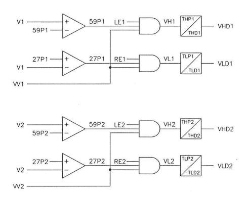
Figure 7: Voltage Control Logic
