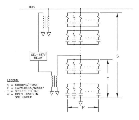
Figure 1: Fused Capacitor Bank With Voltage - Differential Protection
