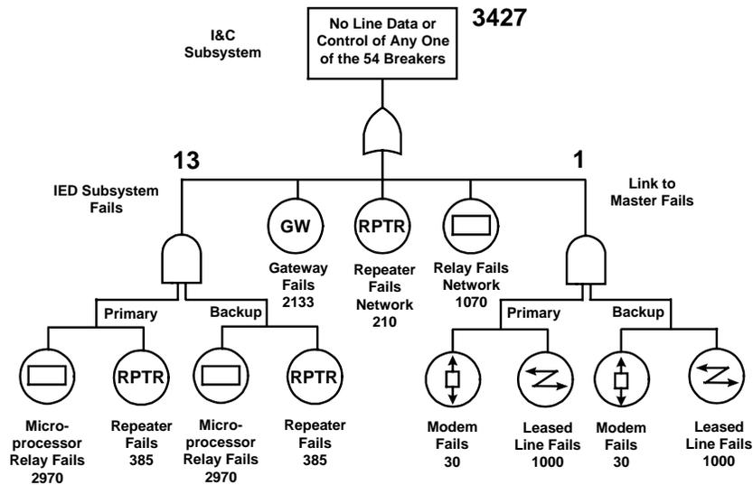
Figure 6: Multidrop Relay Network Centric Westmoreland I&C System
