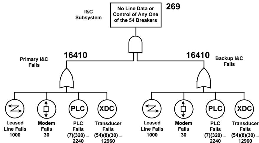
**Figure 4: Fault Tree for PLC Centric Westmoreland I&C System**
