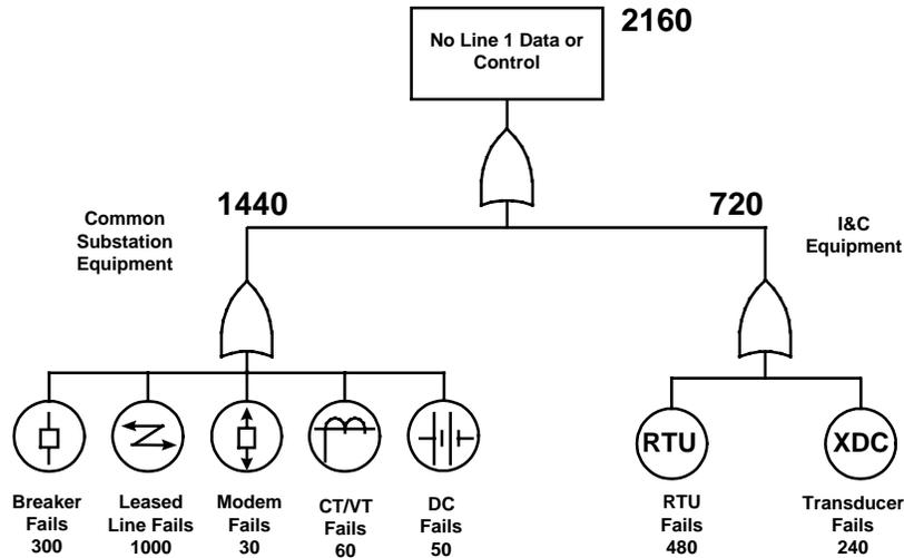
**Figure 1: Fault Tree for RTU-Based I&C System**
