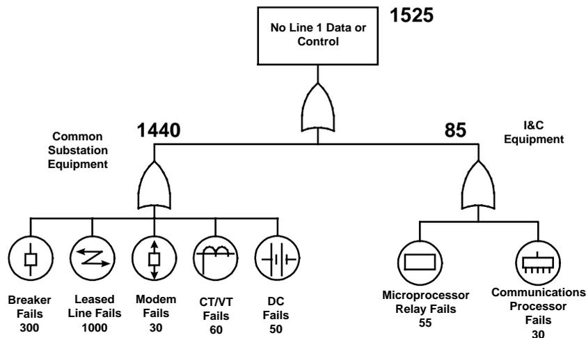
**Figure 2: Fault Tree for Relay and Communications Processor Star I&C System**
