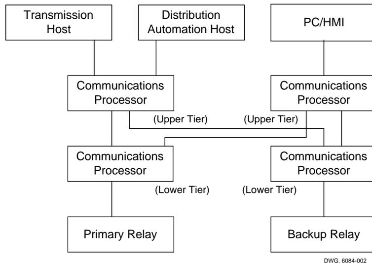
**Figure 9: SI System Two-Tier Architecture**
