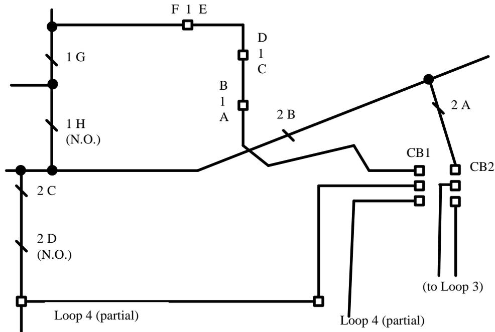
Figure 15: Partial one-line, intelligent switching systems. Overhead team 2 serves also as alternate source for team 1; underground Loop 4 provides the alternate source for team 2.
