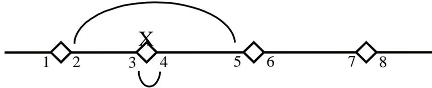
Figure 13: Bus Fault Tripping Scenario; “X” indicates the fault location.
