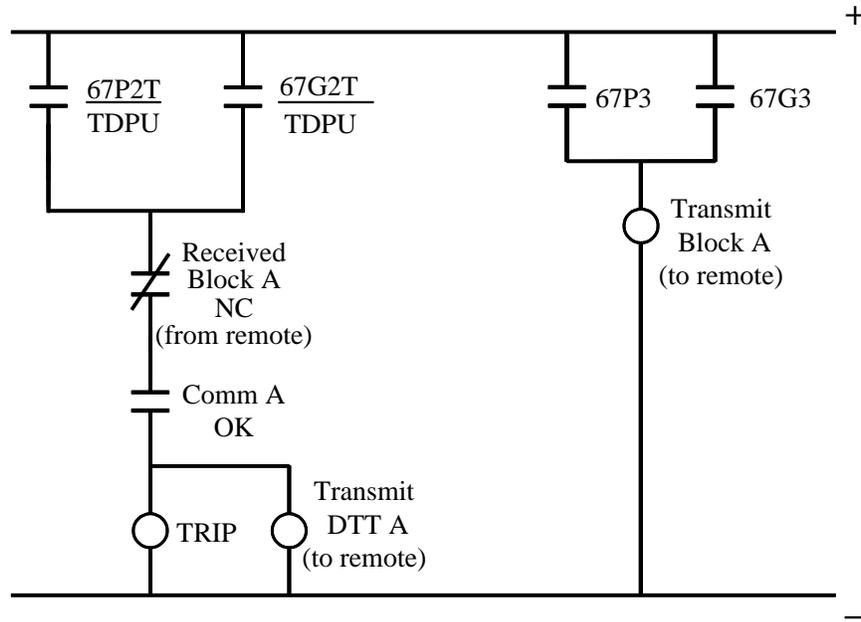
Figure 6: Control circuit representation of DCB logic
