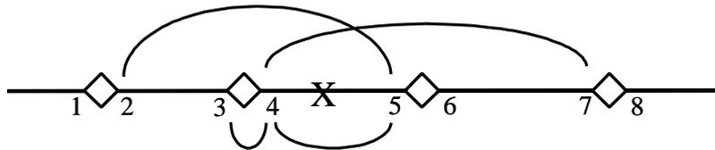
Figure 10: Tripping scenarios for Breaker Failure Scheme; “X” indicates the fault location.
