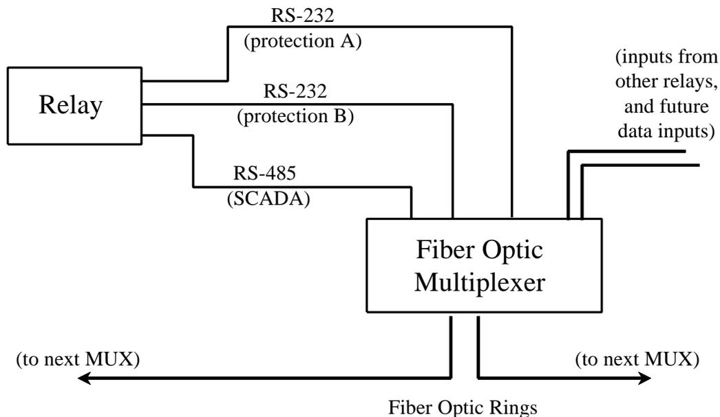
Figure 2: Connection of Relay to the Fiber Optic Communications Network
