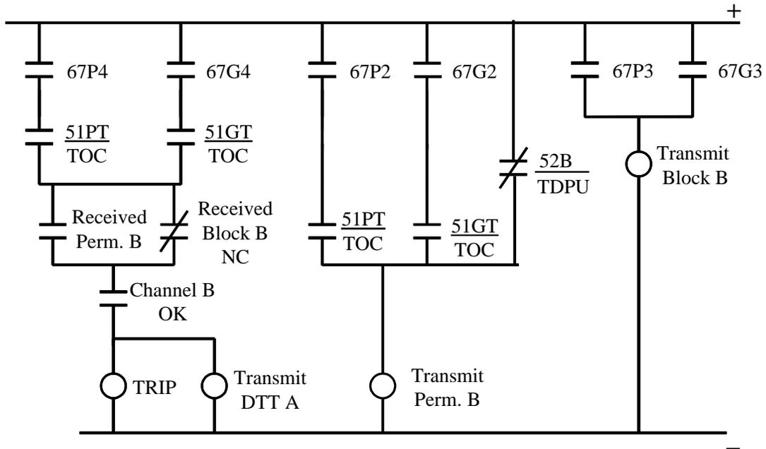
Figure 8: Control circuit representation of Overreaching POTT/DCB Scheme
