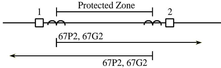
Figure 3: Basic POTT Scheme Protection
