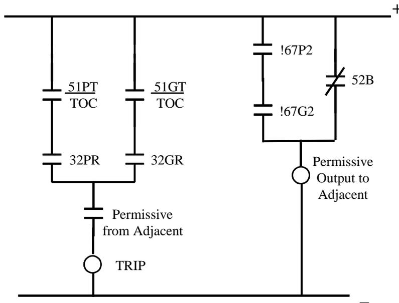
Figure 12: Control circuit representation for Bus Fault logic
