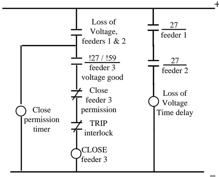
Figure 14: Control circuit representation of Automatic Source Transfer logic.
