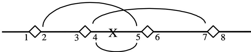
Figure 7: Tripping scenarios for Overreaching POTT/DCB Scheme; “X” indicates the fault location.
