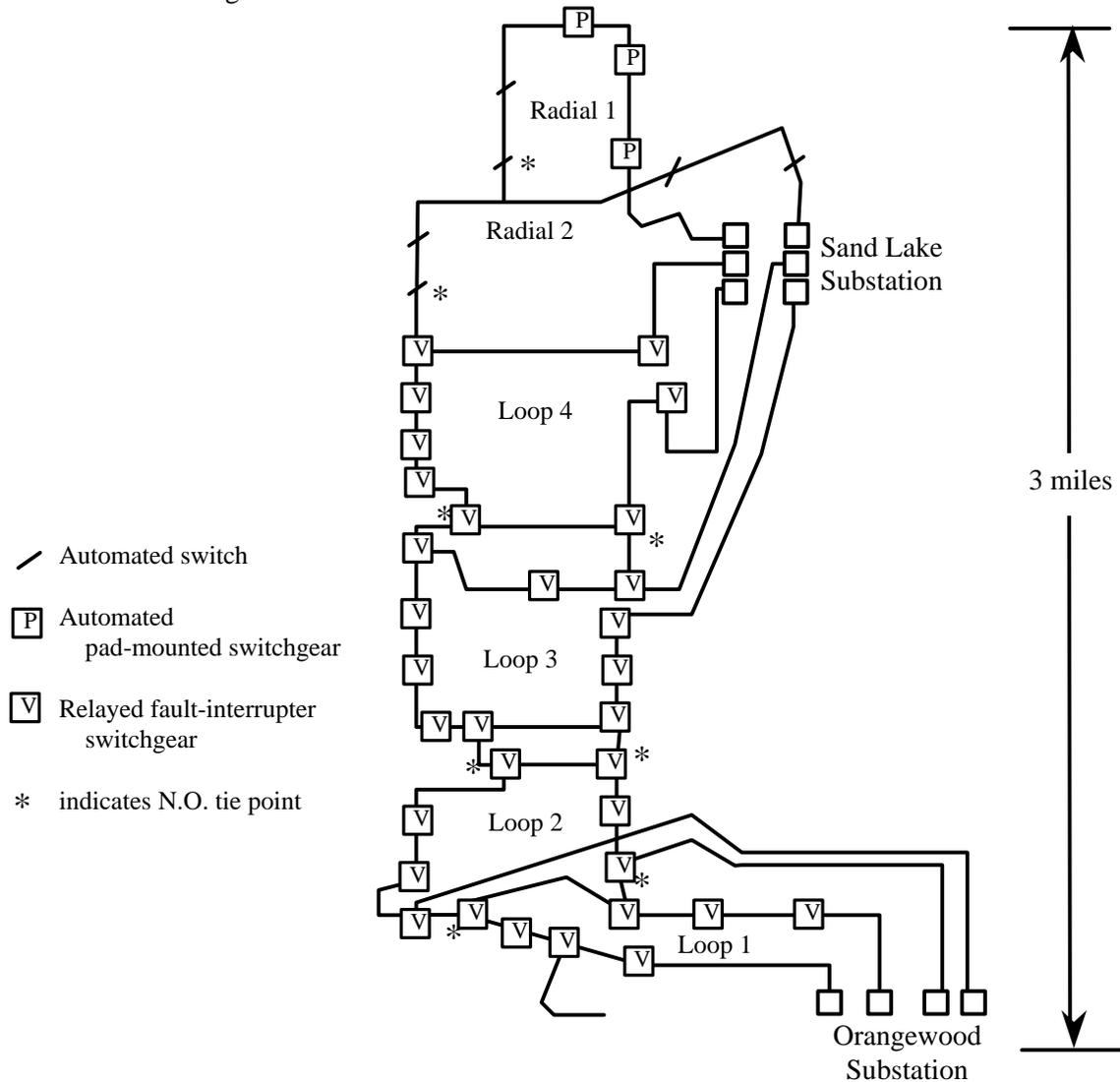
Figure 1: I-Drive Project Distribution System feeders. Branch lines to loads are not shown.
