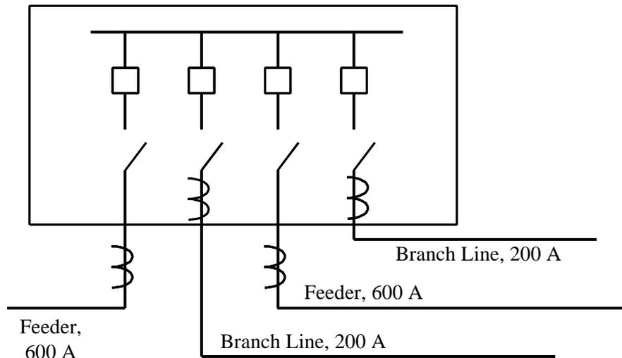
Figure 11: Switchgear one-line showing 600-amp Feeders and 200-amp Branch Lines
