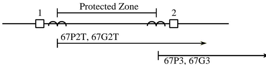
Figure 5: Basic DCB Scheme Protection
