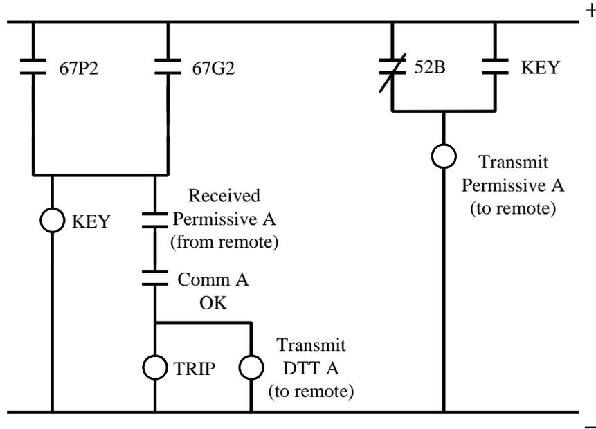
Figure 4: Control circuit representation of POTT logic
