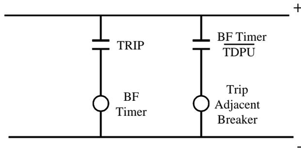
Figure 9: Control circuit representation of Breaker Failure Scheme
