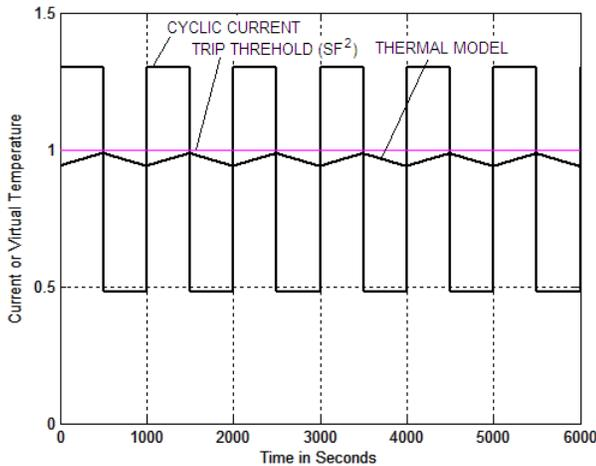
Fig. 4 Response of the Thermal Model to Cyclic Overload
