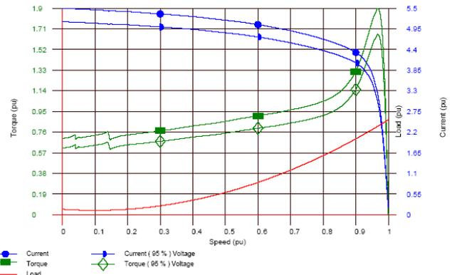
Fig. 2 Current and Torque versus Speed for the WEG 1600 kW Induction Motor
