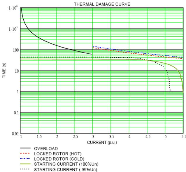
Fig. 1 Thermal Damage Curve for WEG 6600V, 1600 kW, 1000rpm Induction Motor
