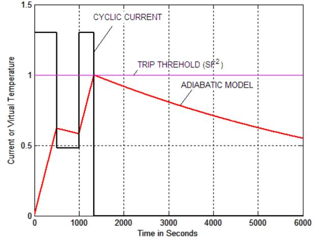
Fig. 5 Response and Premature Trip of the Overcurrent Relay to Cyclic Overload.
