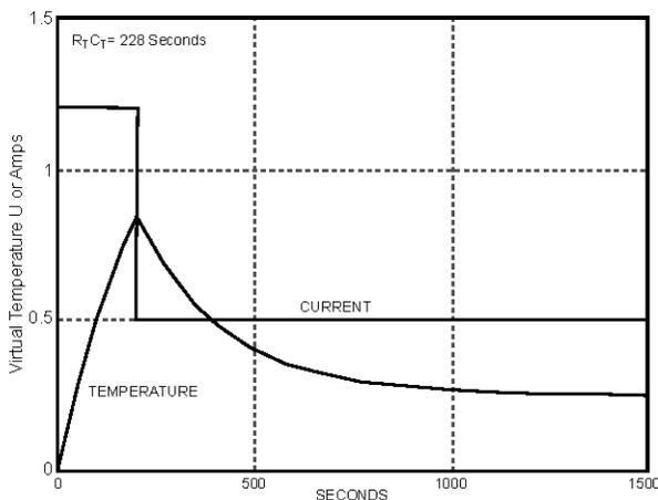
Fig. 6 Dynamic Response of the First Order Thermal Model
