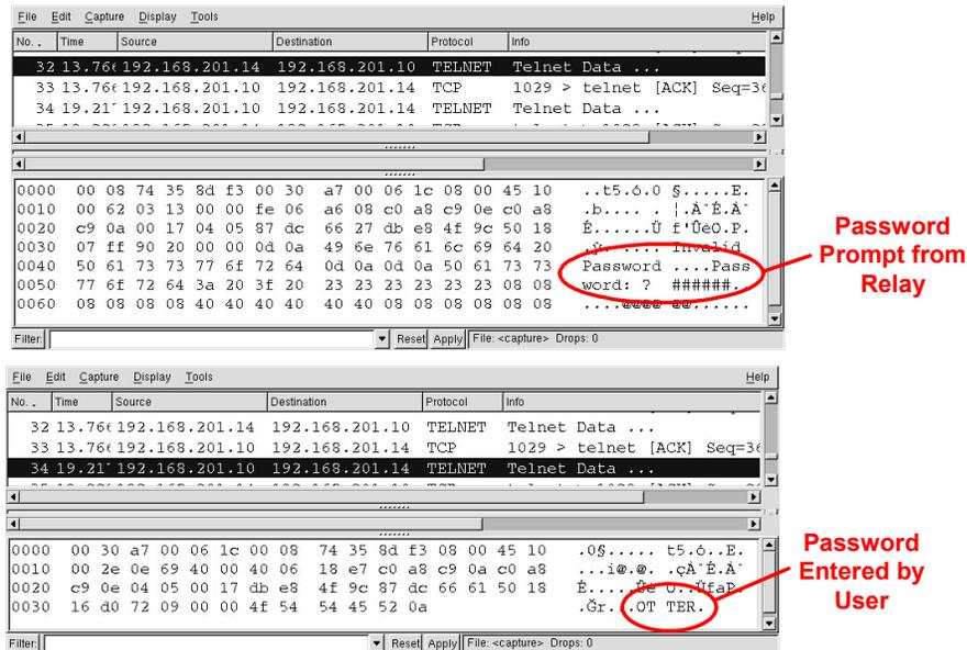
**Figure 4** Figure Showing Electronic Capture of Unencrypted Passwords
