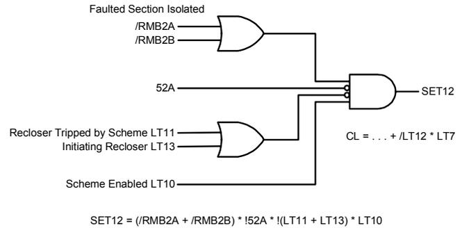
Fig. 8. Scheme Close Logic
