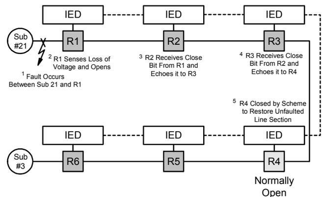
Fig. 11. Scheme Operation for Fault on Sub #21–R1
