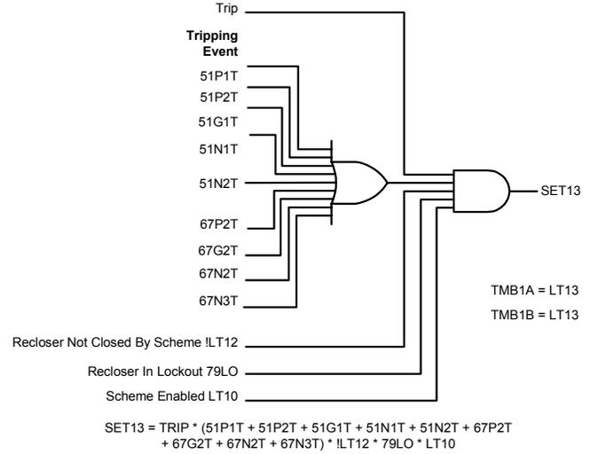
Fig. 4. Scheme Initiate Logic
