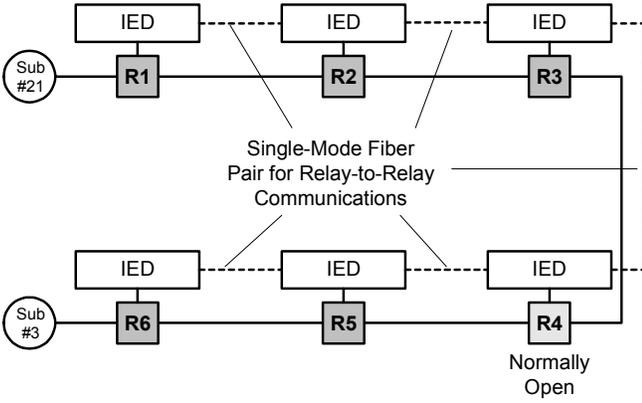
Fig. 2. Communications Diagram
