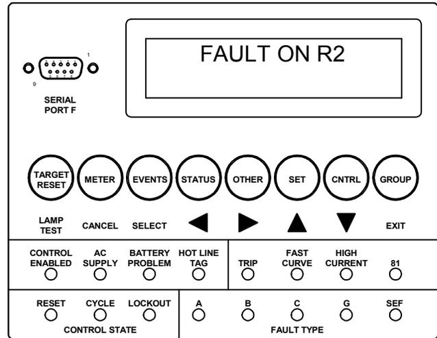
Fig. 13. Display Message Following Operation
