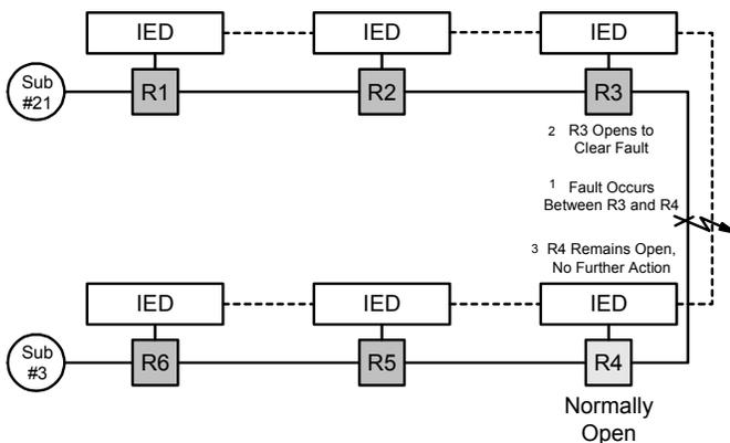
Fig. 10. Scheme Operation for Fault on R3–R4
