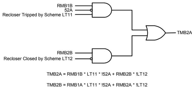
Fig. 7. Close Bit Transmit Logic
