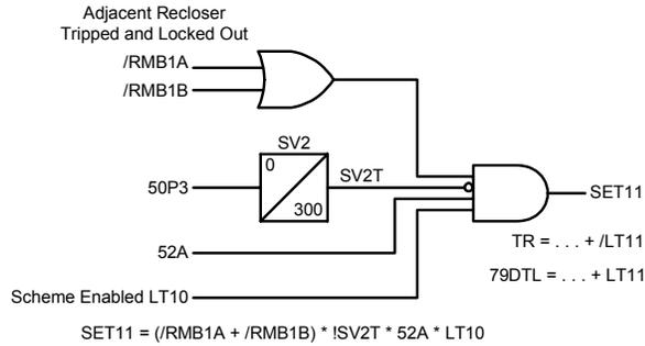
Fig. 5. Scheme Trip Logic for R2–R5
