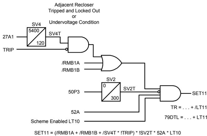
Fig. 6. Scheme Trip Logic for R1 and R6
