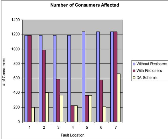
Fig. 14. Number of Customers Subjected to Extended Outage for Faults at Various Points Along the Feeders
