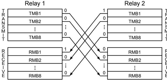
Fig. 3. Relay-to-Relay Communications Representation
