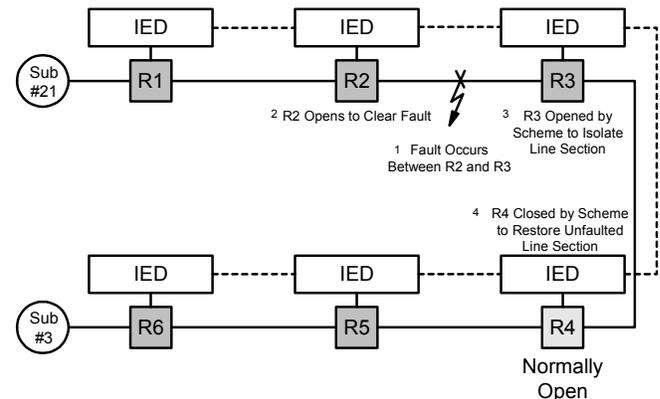
Fig. 9. Scheme Operation for Fault on R2–R3
