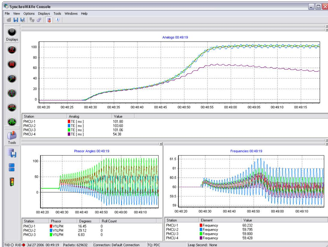
Fig. 5. Unstable Time Error, Phase Angle, and Frequency Following a Fault
