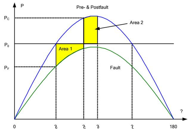
Fig. 8. Clearing Time for Transiently Stable System
