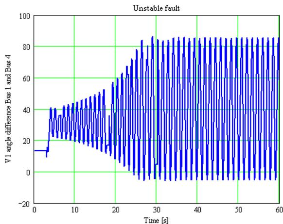
Fig. 9. Positive-Sequence Angle Difference Between Bus 1 and Bus 4
