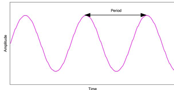
Fig. 1. Measuring Time Error Using a Periodic Waveform
