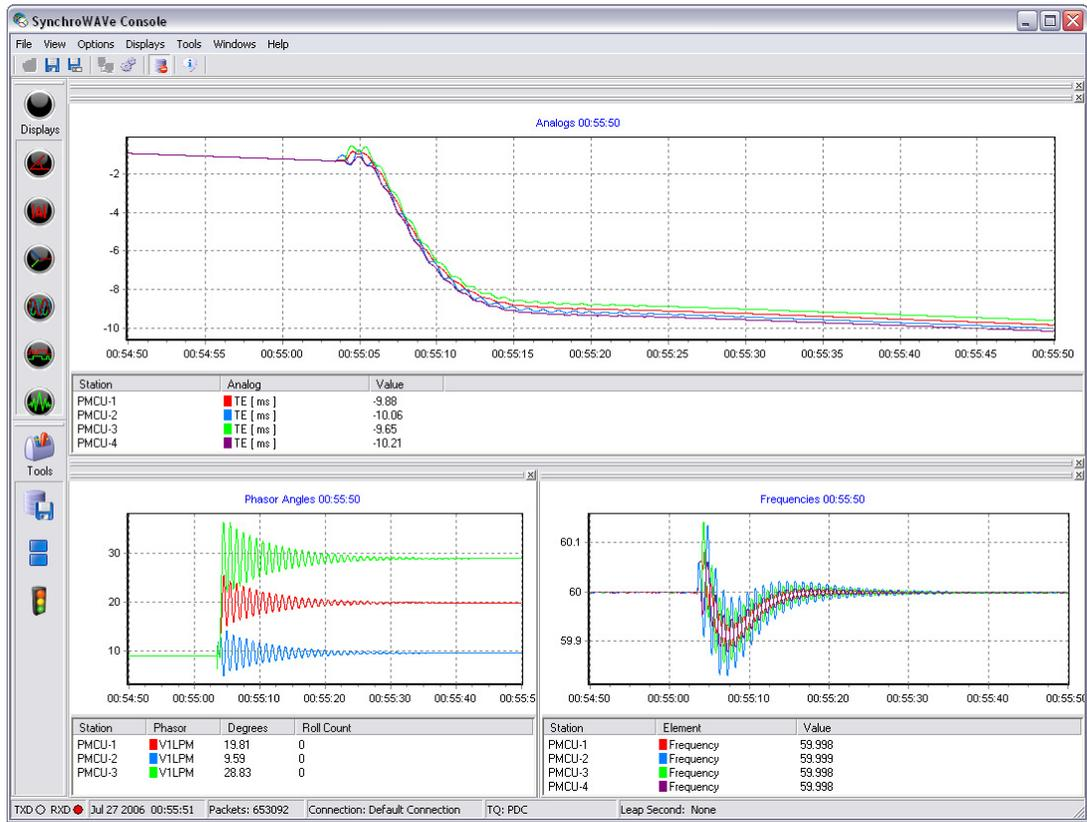
Fig. 4. Stable Time Error, Phase Angle, and Frequency Following a Fault
