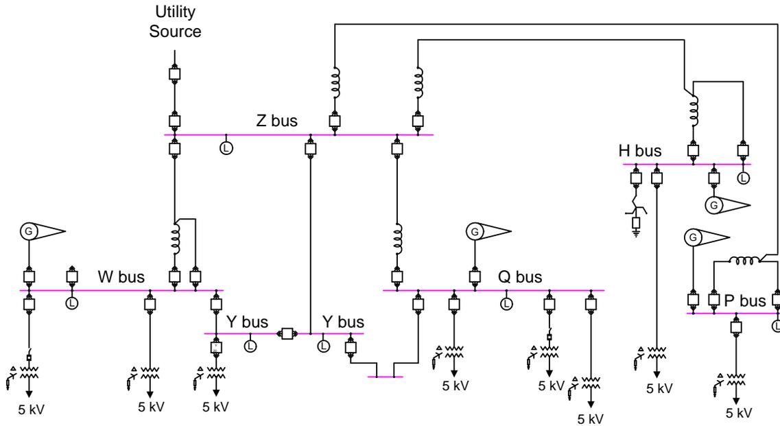
Fig. 1. 15 kV power plant system one-line diagram
