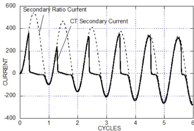
Fig. 8. Current waveforms of a C100, 1200:5 CT, burden 0.5 ohms, 50 kA, X/R equals 17
