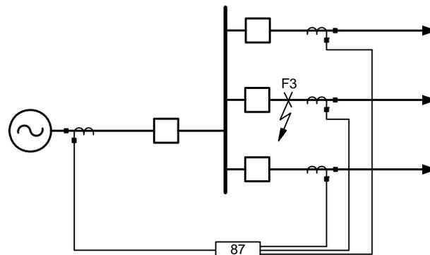
Fig. 9. Low-impedance bus differential scheme showing an end-zone fault, F3, between the breaker and CT
