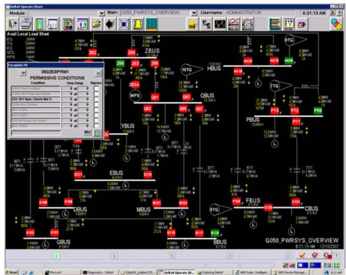
Fig. 4. HMI screen for a 15 kV and 5 kV system with an informational breaker popup window
