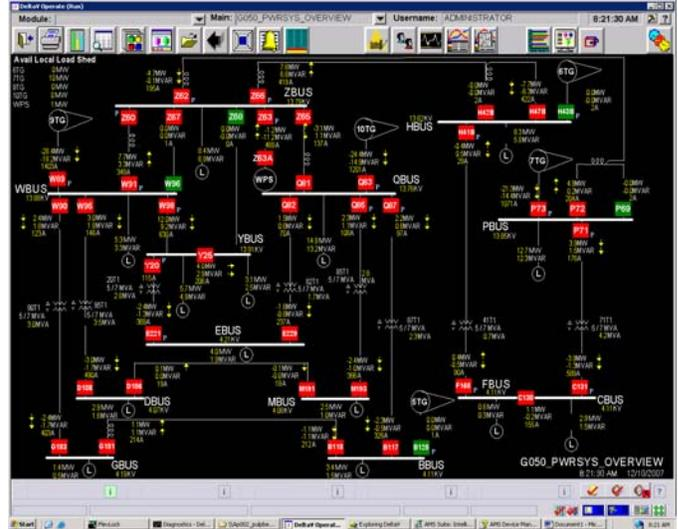
Fig. 3. HMI screen for a 15 kV and 5 kV system
