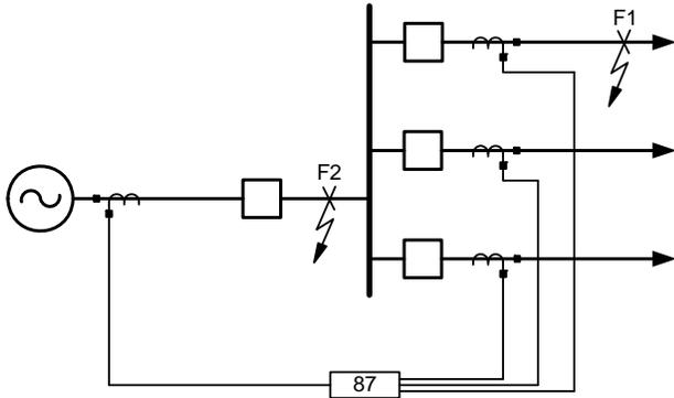
Fig. 6. Low-impedance bus differential scheme showing an external fault, F1, and an internal fault, F2
