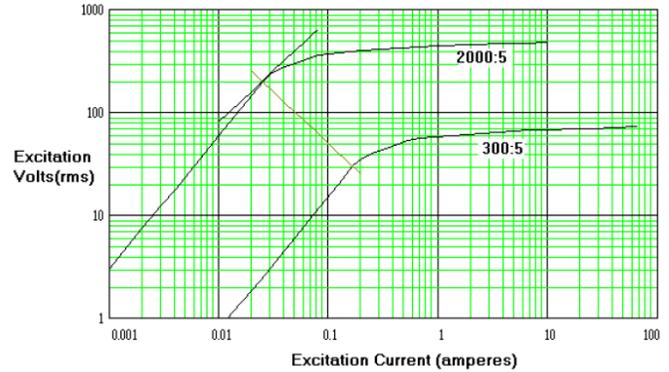
Fig. 7. 2000:5 CT excitation curve and its 300:5 tap, both with knee-point tangents and normal lines
