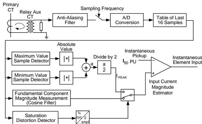
Fig. 12. Instantaneous element using the cosine-peak adaptive filter
