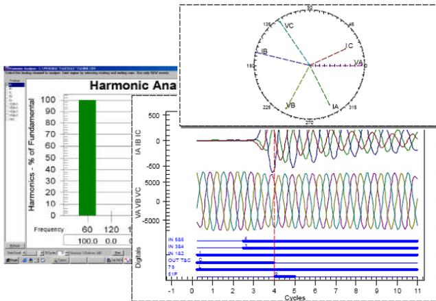
Fig. 13. Software tools convert numerical event report data into graphical plots and charts
