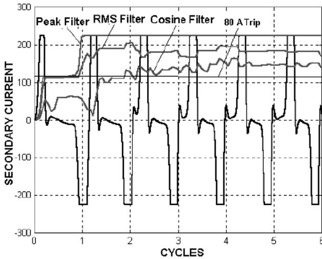
Fig. 11. Filter response, fault 40 kA, X/R equals 20, C100, 200:5 CT, 0.5  $\Omega$  burden
