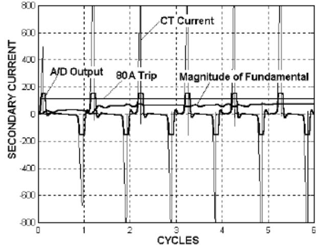
Fig. 10. CT and relay signals for a 40 kA fault using C50, 100:5 CTs
