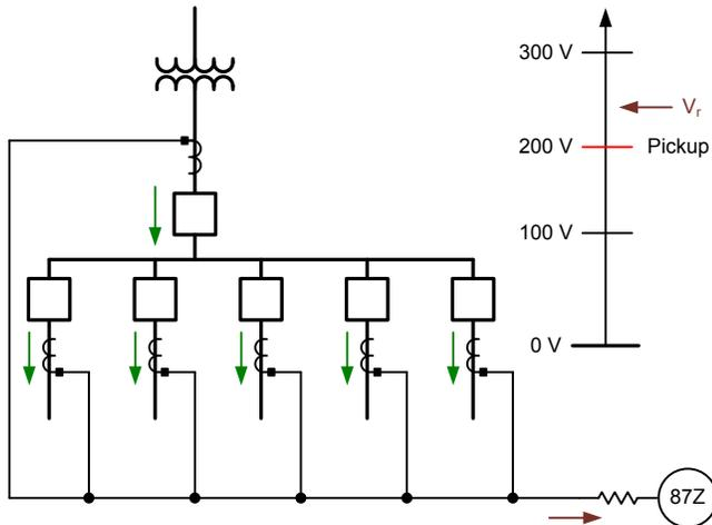
Fig. 25. Example one-line diagram with an open CT connection
