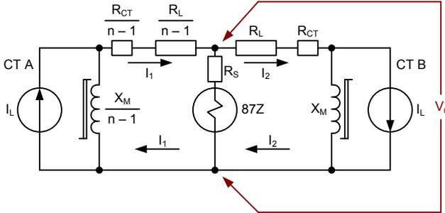
Fig. 13. Equivalent two-CT circuit showing balanced current in parallel CTs
