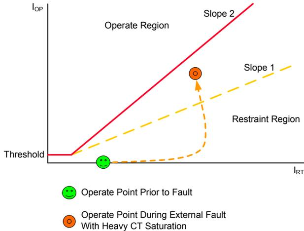
Fig. 7. High-security bus differential relay characteristic
