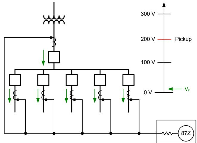
Fig. 14. Balanced current flow in CTs for through-load condition
