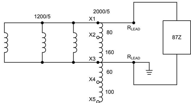
Fig. 28. Mismatched CT connection using the matching tap of the higher ratio CT
