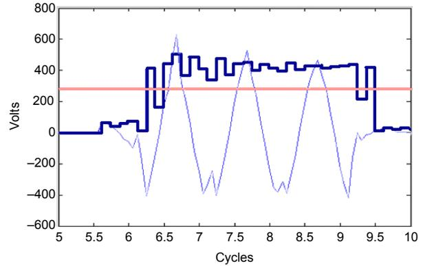
Fig. 20. One-half-cycle cosine filtered output (thin blue line), the magnitude of the output (thick blue line), and the relay 200 V trip threshold (peak of setting shown with red line)
