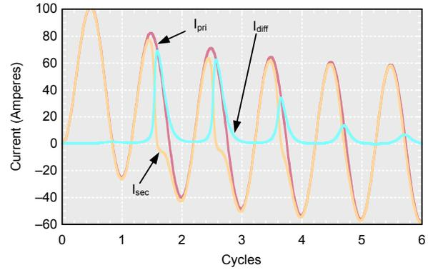
Fig. 5. Saturated CT secondary current and resulting difference current,  $I_{diff}$
