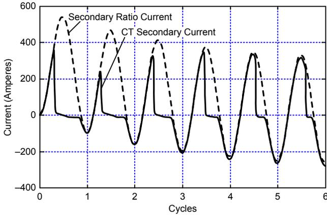
Fig. 9. Current waveforms of a C100, 1200:5 CT with burden of 0.5 ohms, 50 kA, and X/R equal to 17
