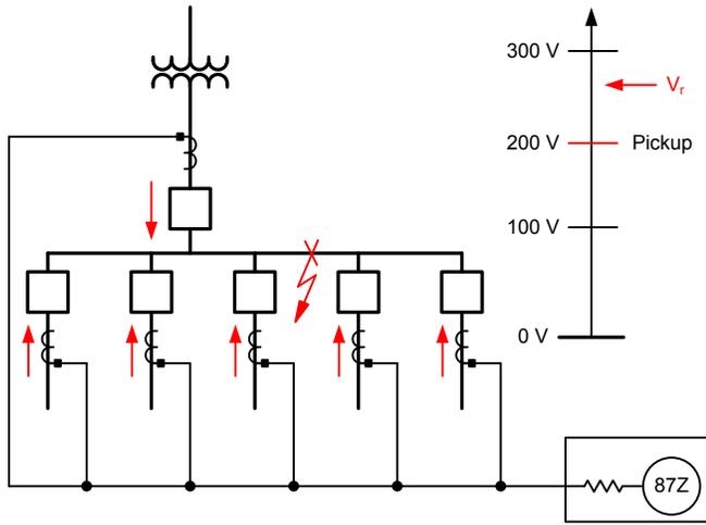
Fig. 18. Fault current flow for an internal bus fault
