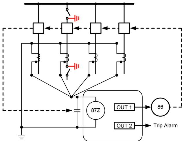
Fig. 27. Grounding chains during breaker maintenance can disable or desensitize a high-impedance bus differential relay
