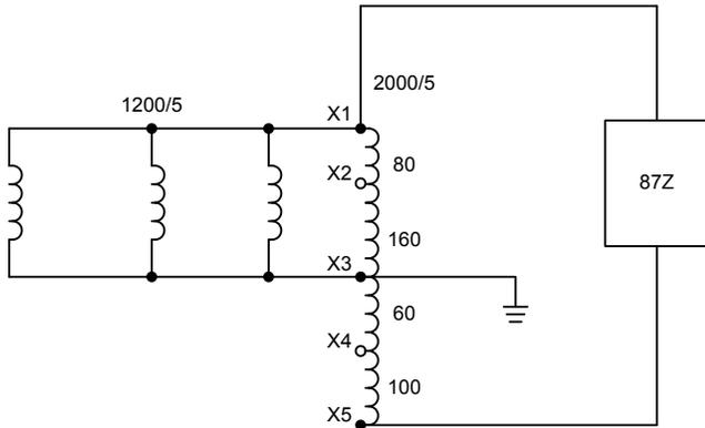
Fig. 29. Mismatched CT connection using the full ratio tap of the higher ratio CT connected to the high-impedance relay
