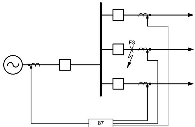
Fig. 8. Low-impedance bus differential scheme showing an end-zone fault, F3, between the breaker and CT
