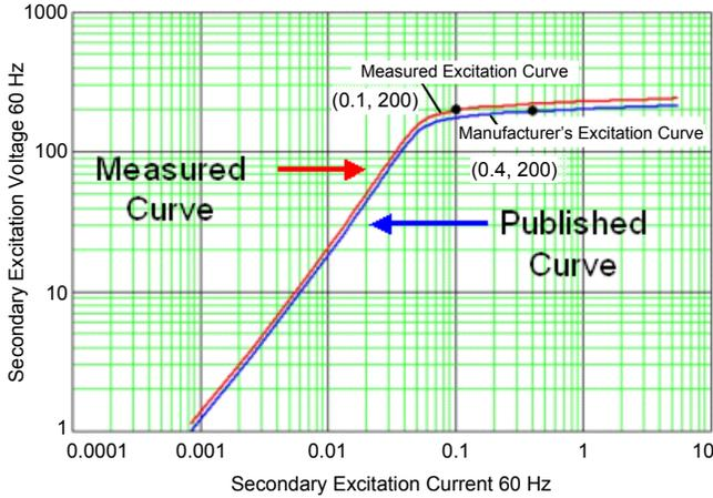
Fig. 23. Measured and published excitation current characteristics for a 1200/5, C200 class CT with a relay pickup voltage threshold of 200 V
