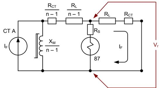
Fig. 15. Equivalent two-CT circuit showing effects of complete saturation on the fault circuit
