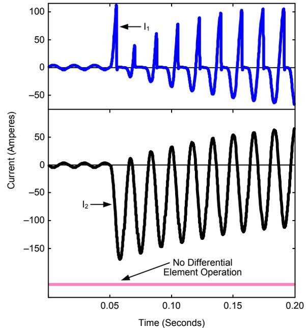
Fig. 6. The relay securely avoids tripping even with severe CT saturation
