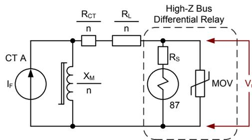
Fig. 17. Equivalent circuit of  $n$  CTs driving current into the high-impedance bus differential relay during an internal bus fault
