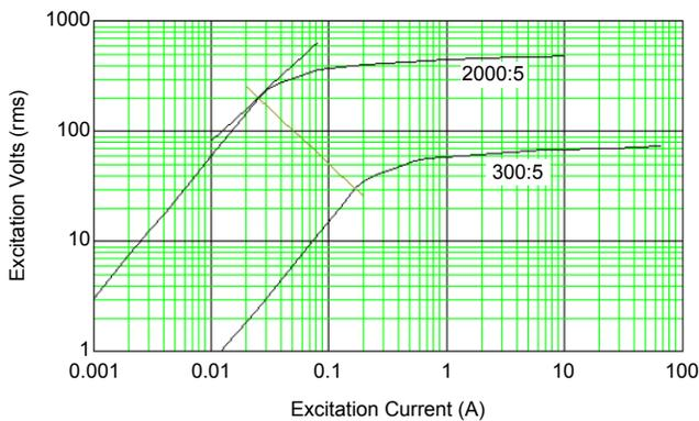
Fig. 10. 2000:5 CT excitation curve and its 300:5 tap, both with knee-point tangents and normal lines
