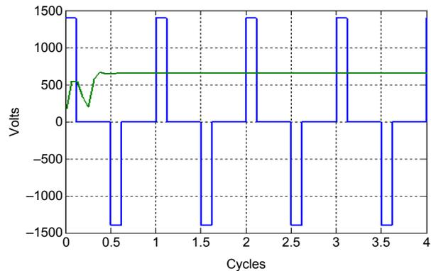
Fig. 21. Voltage waveform and filtered output magnitude for a 60 kA primary current through a 1200/5, C400 class CT connected to a high-impedance bus differential relay with a 1400 V MOV
