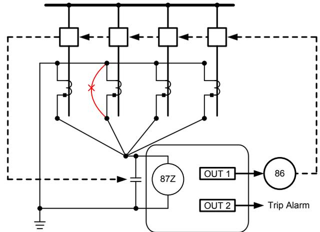
Fig. 26. Shorted CT disables high-impedance bus differential relay
