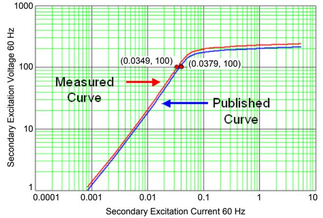
Fig. 22. Measured and published excitation current characteristics for a 1200/5, C200 class CT with a relay pickup voltage threshold of 100 V
