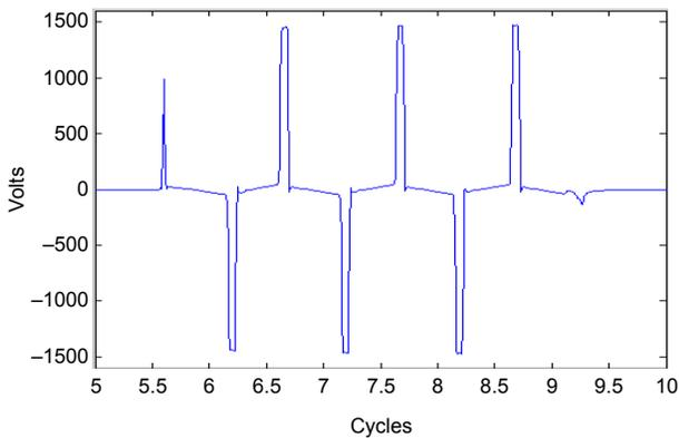
Fig. 19. Voltage waveform for a 60 kA primary current through a 1200/5, C200 class CT connected to a high-impedance bus differential relay with a 1400 V MOV
