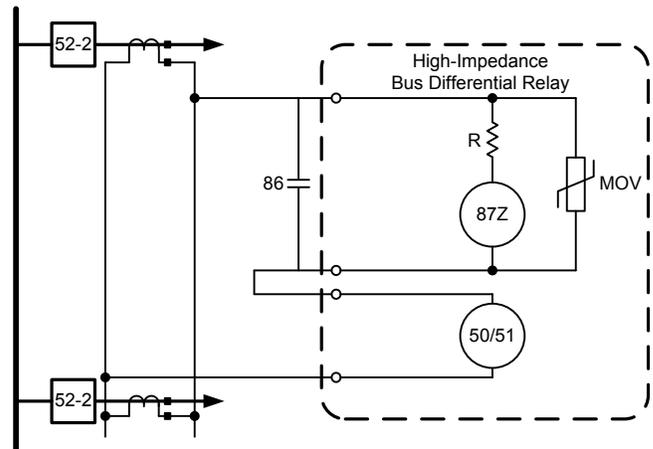
Fig. 12. High-impedance bus differential relay internal elements
