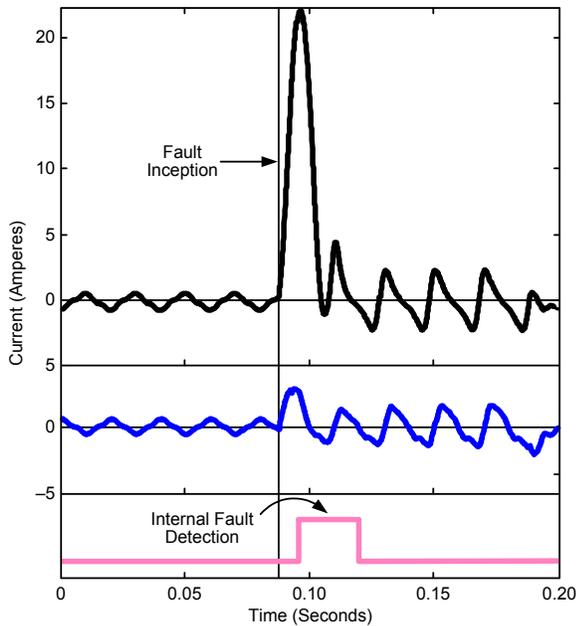
Fig. 4. Subcycle relay operation for an internal bus fault
