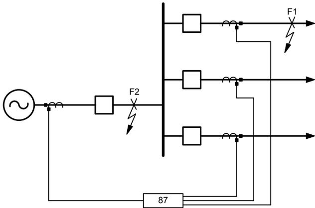
Fig. 2. Low-impedance bus differential scheme showing an external fault, F1, and an internal fault, F2
