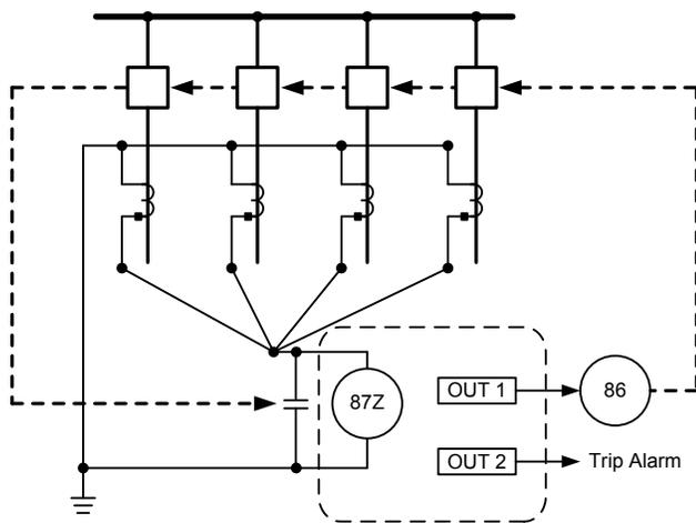
Fig. 11. Paralleled CTs connected to a high-impedance bus differential relay
