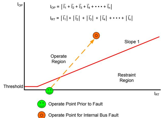
Fig. 3. Percentage current differential characteristic of a low-impedance bus differential relay with and without an internal bus fault
