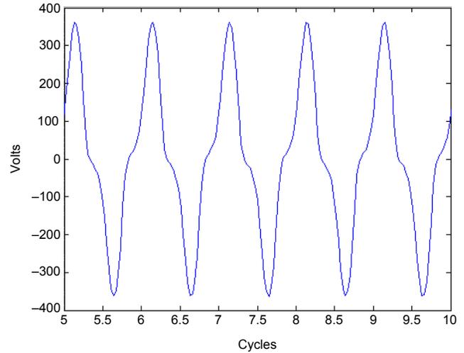
Fig. 24. Voltage waveform at the 200 V pickup point with C200 rated CTs
