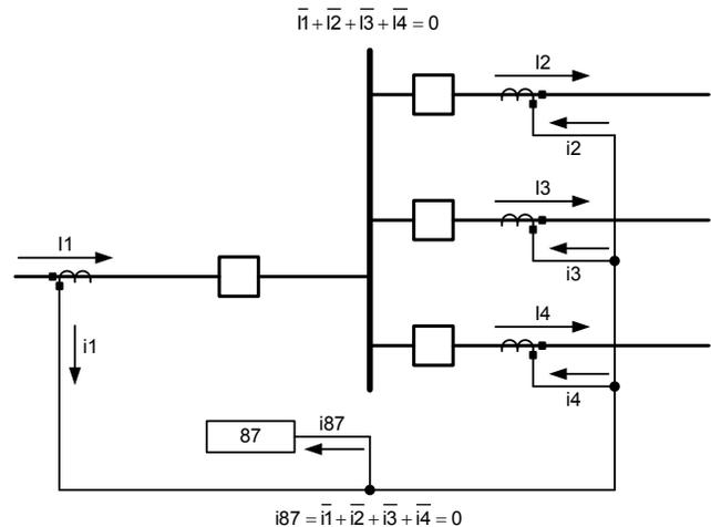
Fig. 1. Simple current differential scheme with paralleled CTs
