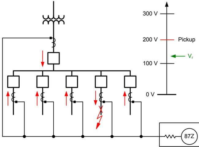
Fig. 16. Fault current flow for an external bus fault
