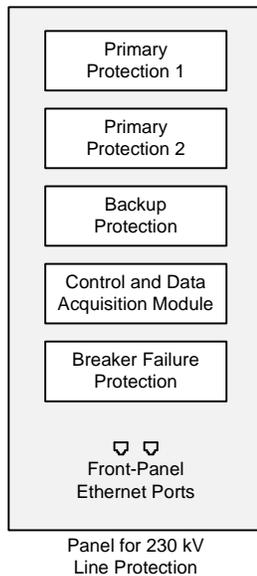
Fig. 12. Ethernet connection points on the front panel
