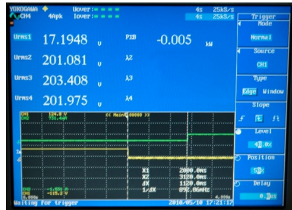
Fig. 13. Live system islanding event results
