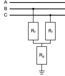
Fig. 10. Fault resistances for a Phase-B-to-Phase-C fault
