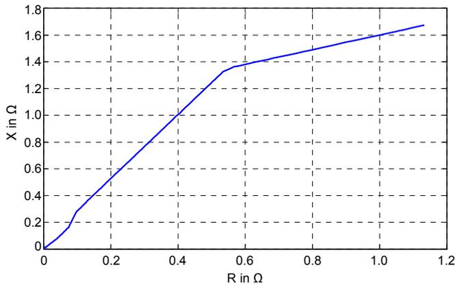
Fig. 3. Distribution feeder positive-sequence impedance is nonhomogeneous
