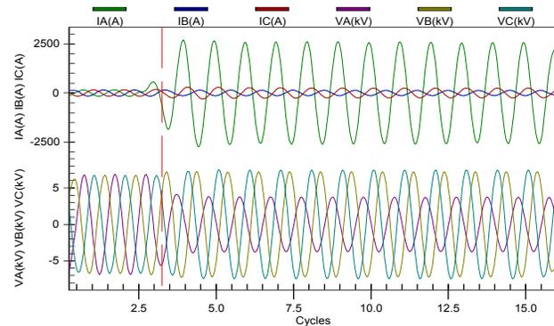
Fig. 18. Recorded fault voltages and currents for a phase-to-ground fault at the end of Section FD00055
