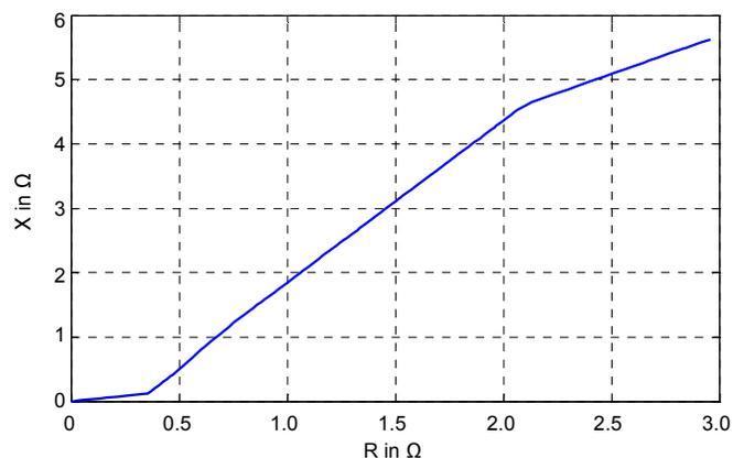
Fig. 4. Distribution feeder zero-sequence impedance is nonhomogeneous
