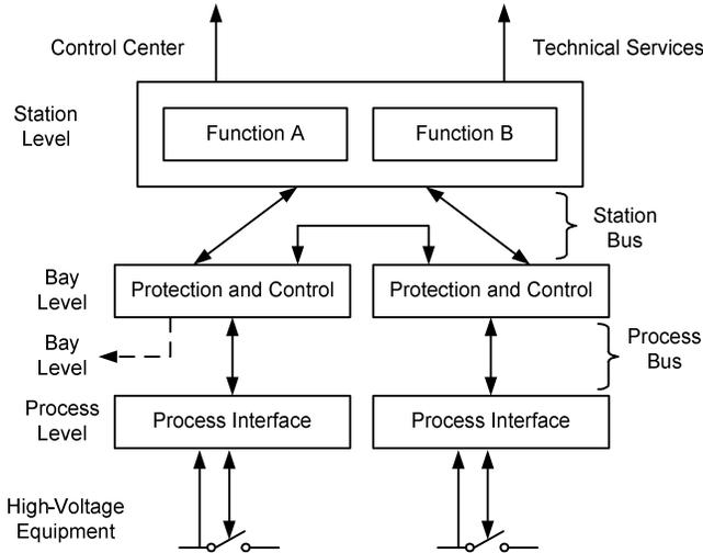
Fig. 5. Structure of substation automation system (SAS).
