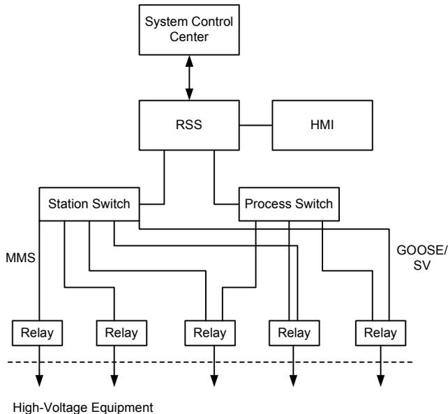
Fig. 11. Decentralized protection system for Liang Shuijing substation project.
