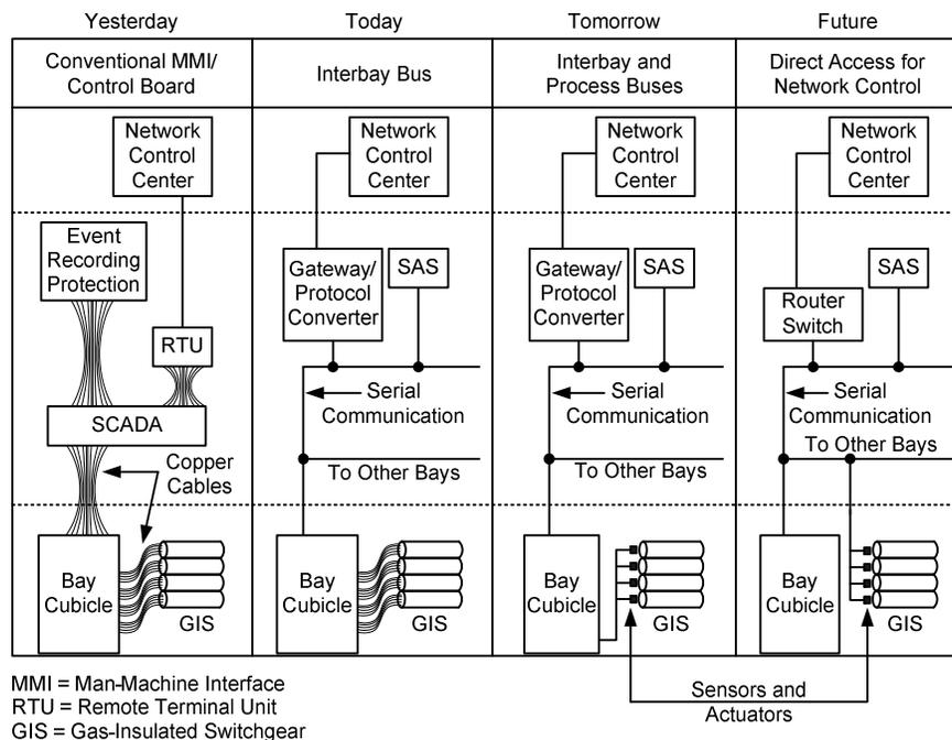
Fig. 7. The developing trend of SASs.
