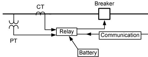
Fig. 1. Schematic diagram of protection system.
