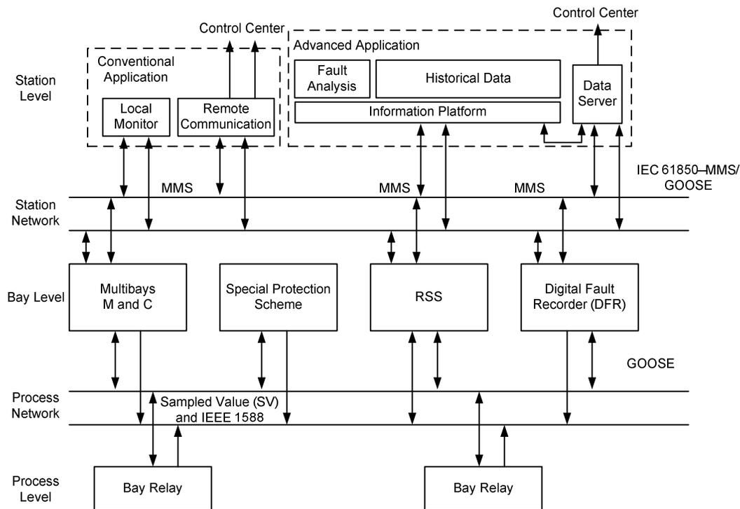
Fig. 8. Innovative RSS architecture based on IEC 61850.
