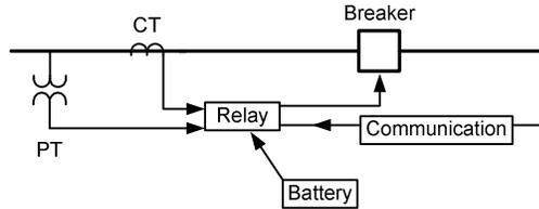
Fig. 1. Schematic diagram of protection system.
