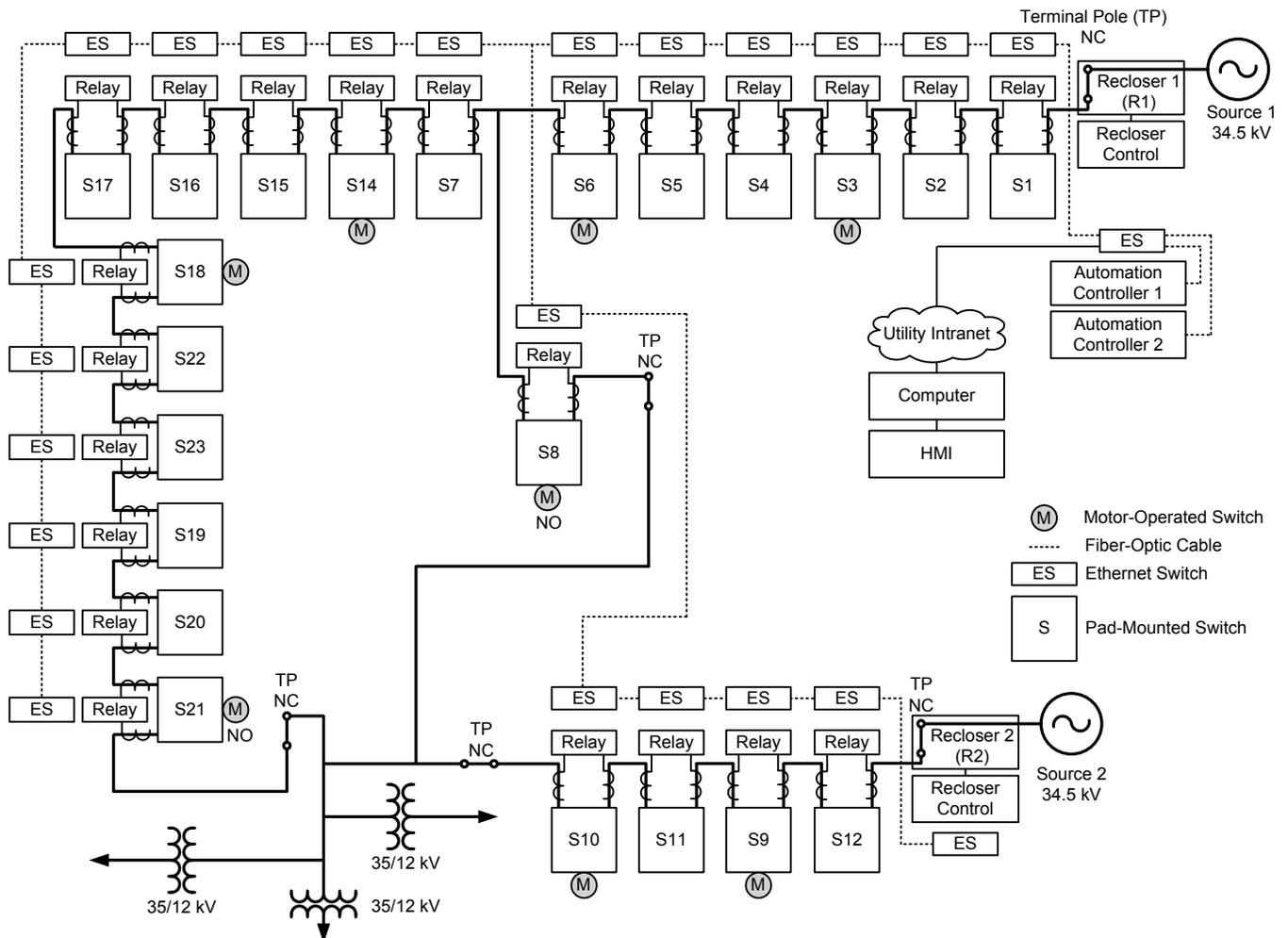
Fig. 1. The UDAS Architecture
