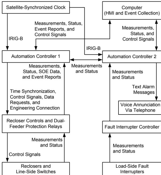
Fig. 2. System Information Flow Diagram
