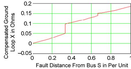
Fig. 7. Compensated ground loop reactance ( $k_0 = 0.66\angle 0^\circ$ ).
