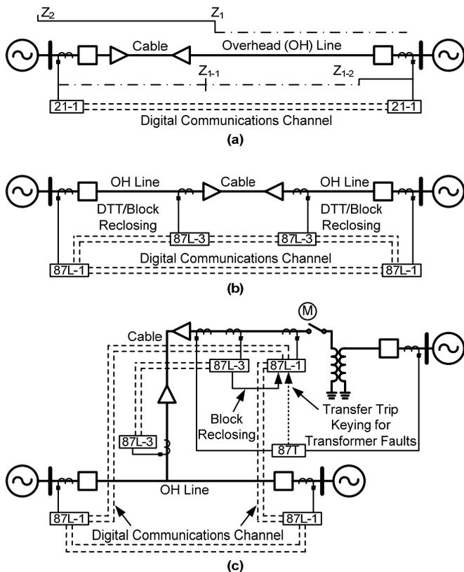
Fig. 9. Mixed overhead and underground circuits.
