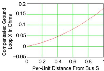
Fig. 5. Bus S compensated ground loop reactance ( $k_0 = 0.66\angle 0^\circ$ ).
