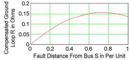
Fig. 6. Compensated ground loop resistance ( $k_0 = 0.66\angle 0^\circ$ ).
