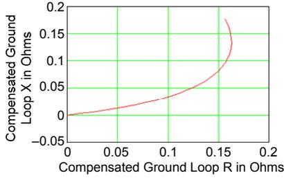
Fig. 2. Bus S compensated ground loop impedance ( $k_0 = 0.66\angle 0^\circ$ ).
