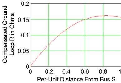
Fig. 4. Bus S compensated ground loop resistance ( $k_0 = 0.66\angle 0^\circ$ ).
