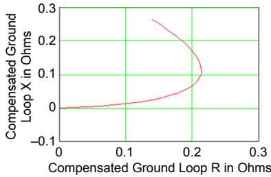
Fig. 3. Bus R compensated ground loop impedance ( $k_0 = 0.66\angle 0^\circ$ ).
