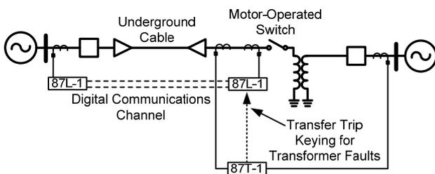
Fig. 8. EHV cable terminated in a transformer.
