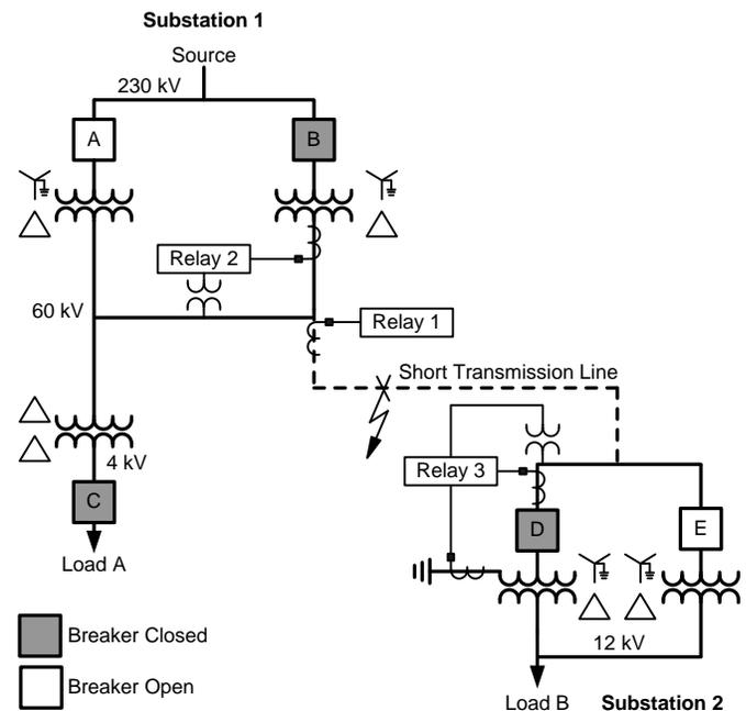
Fig. 9. System Configuration During a Ground Fault
