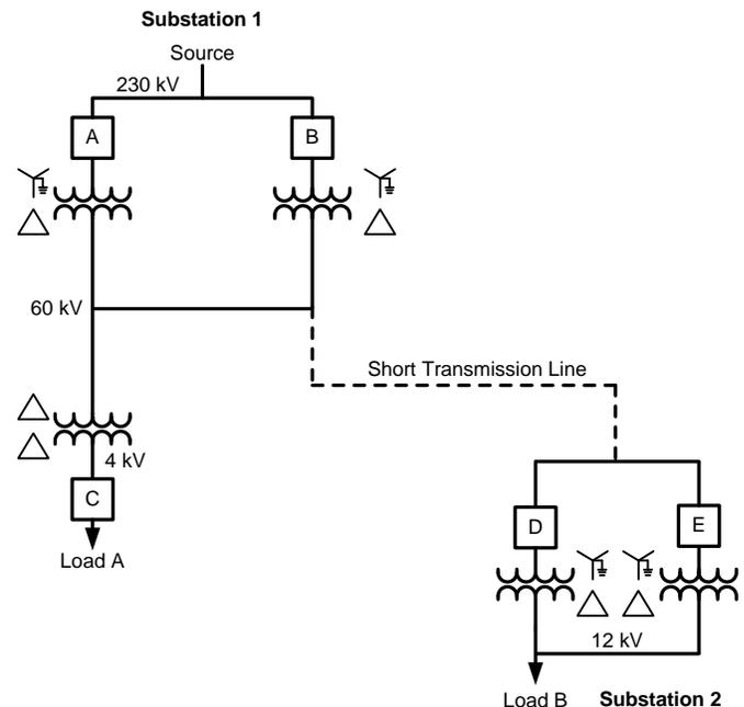
Fig. 4. Portion of the System With Transformer Configurations
