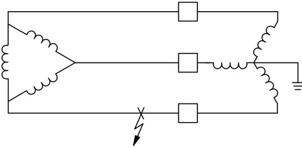
Fig. 18. Zero-Sequence Current Flow With Breaker D Open
