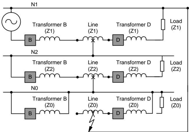
Fig. 15. Sequence Diagram of Single-Phase-to-Ground Fault When Breaker D Is Closed
