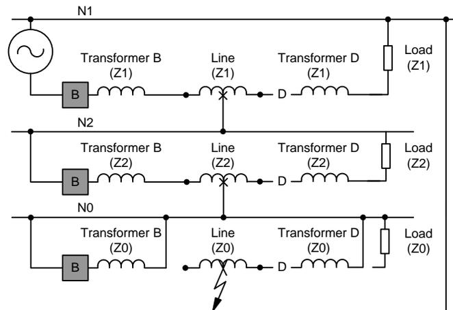
Fig. 17. Sequence Diagram of Fault When Breaker D Is Open
