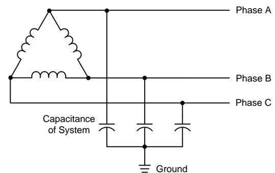
Fig. 1. Line-to-Ground Capacitance of an Ungrounded System
