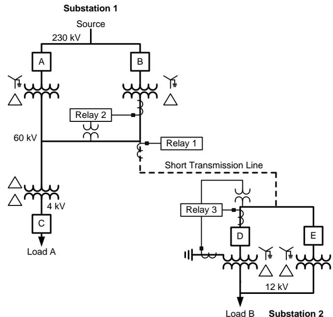
Fig. 6. Relaying Applied to the 60 kV System
