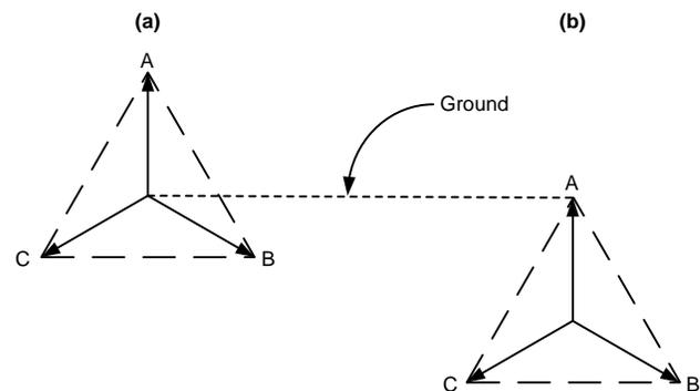
Fig. 2. Voltage Vector Triangle for an Unfaulted System (a) and a System With an SLG Fault (b)
