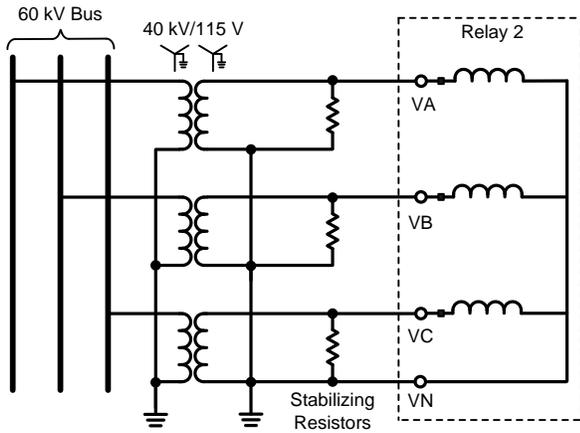
Fig. 7. Four-Wire VT Connection
