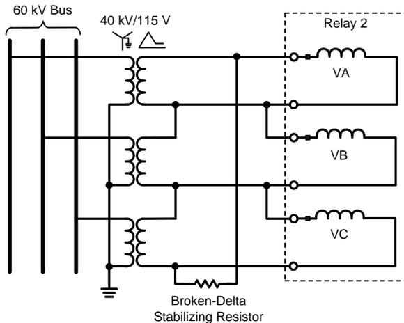
Fig. 8. Relay 2 Six-Wire VT Connection
