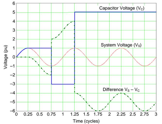
Fig. 3. Transient Overvoltage From a Restriking Ground Fault
