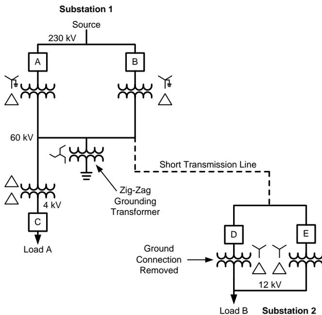
Fig. 5. Implementing a Grounding Transformer
