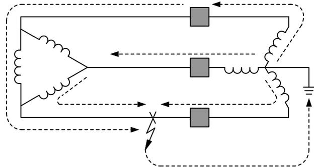
Fig. 16. Zero-Sequence Current Flow With Breaker D Closed
