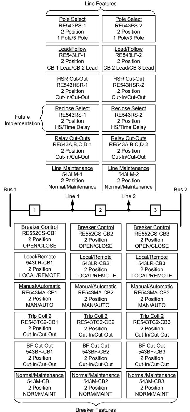
Fig. 6. Operator Interface Switches
