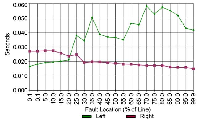
Fig. 9. Zone 2 Maximum Assertion Time for Faults Along the Line
