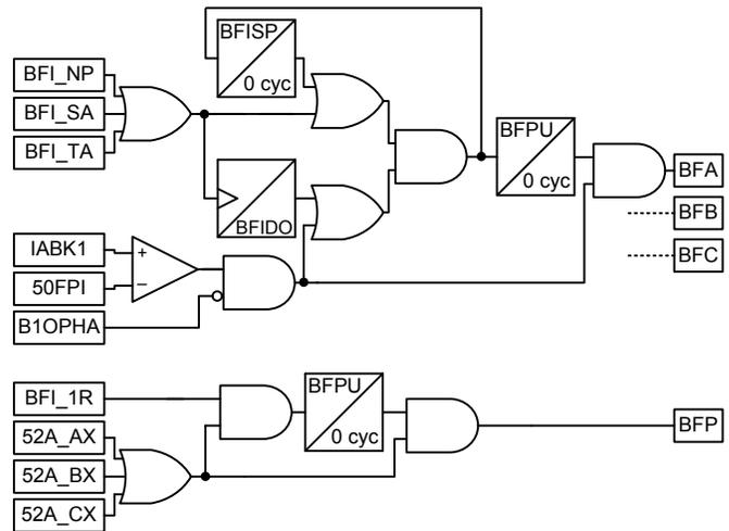
Fig. 5. Custom Breaker Failure Logic
