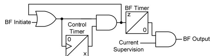
Fig. 13. Original PG&E Breaker Failure Logic
