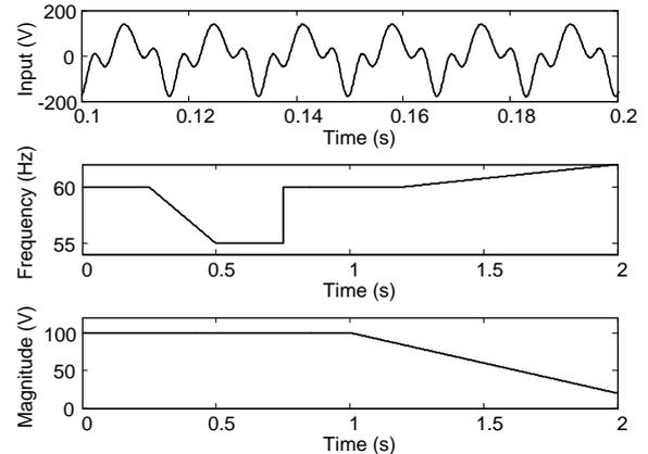
Fig. 3. Input signal used for testing: waveform (top), frequency (middle), and magnitude of fundamental frequency component (bottom).
