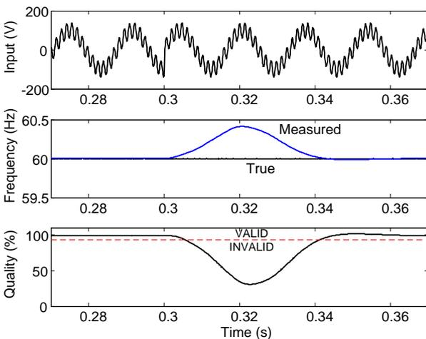
Fig. 6. Response of the new algorithm to a switching event: input waveform (top), frequency (middle), and quality-of-measurement index (bottom).
