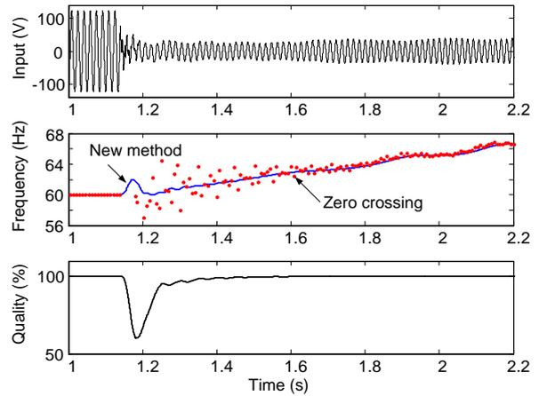
Fig. 7. Transient simulation example including subsynchronous oscillations and a low-inertia generator.
