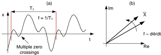
Fig. 1. Frequency measurement methods: zero crossings (a) and rate-of-change of phasor rotation (b).
