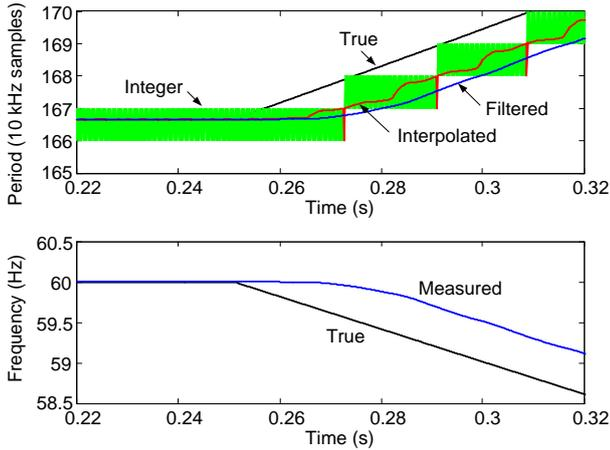
Fig. 4. New algorithm operation illustration: period (top) and frequency (bottom) for a  $-20$  Hz/s ramp.
