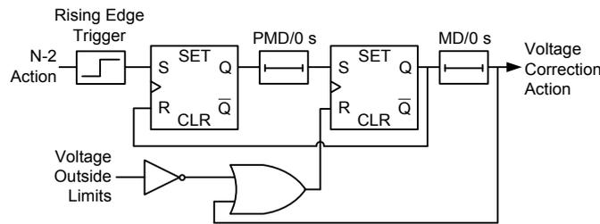
Fig. 6. Voltage correction logic.
