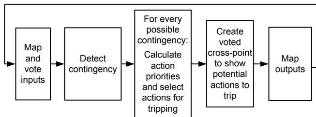
Fig. 4. Core logic diagram.
