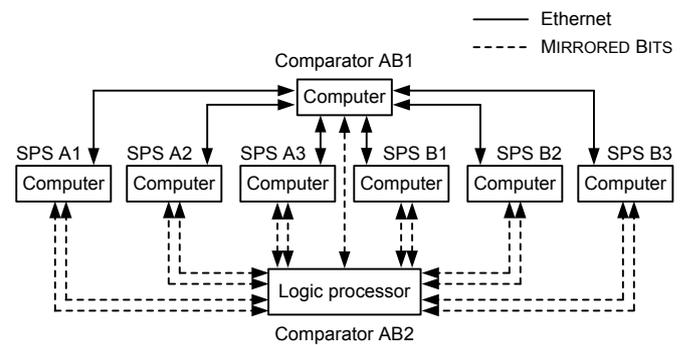
Fig. 1. Triple modular redundant supervisory architecture.
