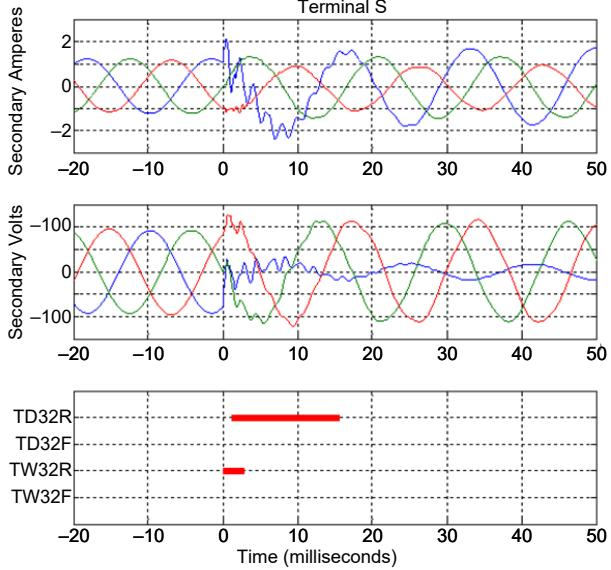
Fig. 12. The time-domain directional elements (TD32 and TW32) on the unfaulted circuit declared the fault shown in Fig. 11 as reverse at Terminal S.
