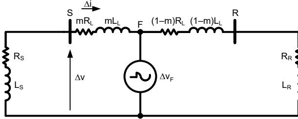
Fig. 3. Fault network of the Fig. 2 system for a fault on the line between Terminal S and Terminal R (a forward fault for a relay at Terminal S).
