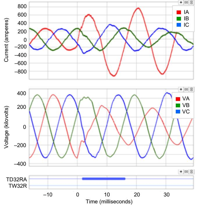
Fig. 32. Currents and voltages captured at TMD and the time domain protection element operation for the external fault on January 15.
