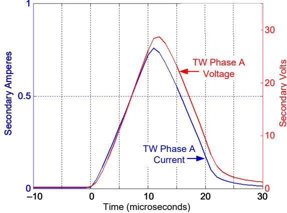
Fig. 15. The TW phase voltage and current of Circuit 2 at Terminal R have the same polarity for the fault shown in Fig. 11.
