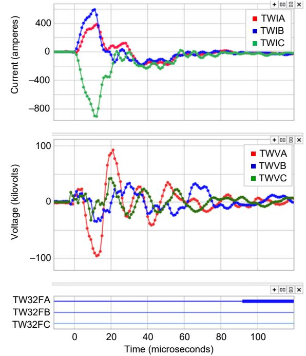
Fig. 29. TW currents and voltages captured at TMD and the TW32 protection element operation for the internal fault on May 4.
