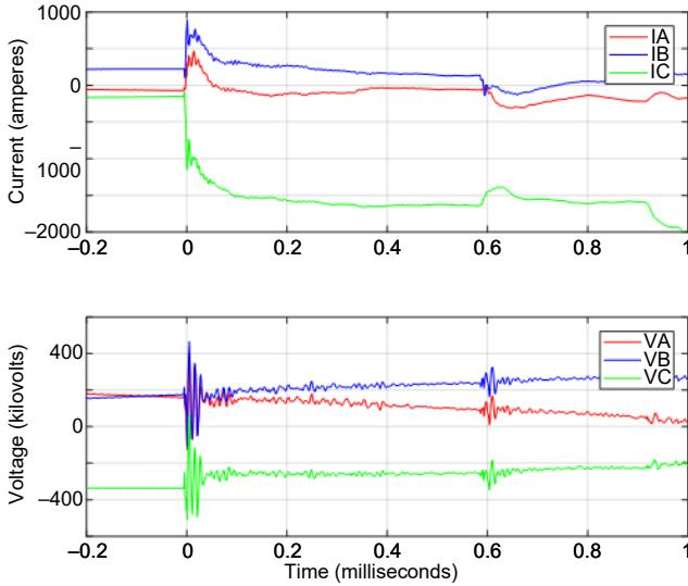
Fig. 20. Fault initiation detail showing the phase currents and the high-frequency voltage information supplied by the CCVTs.
