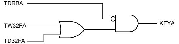
Fig. 16. Key transmitter logic for accelerating the POTT scheme.
