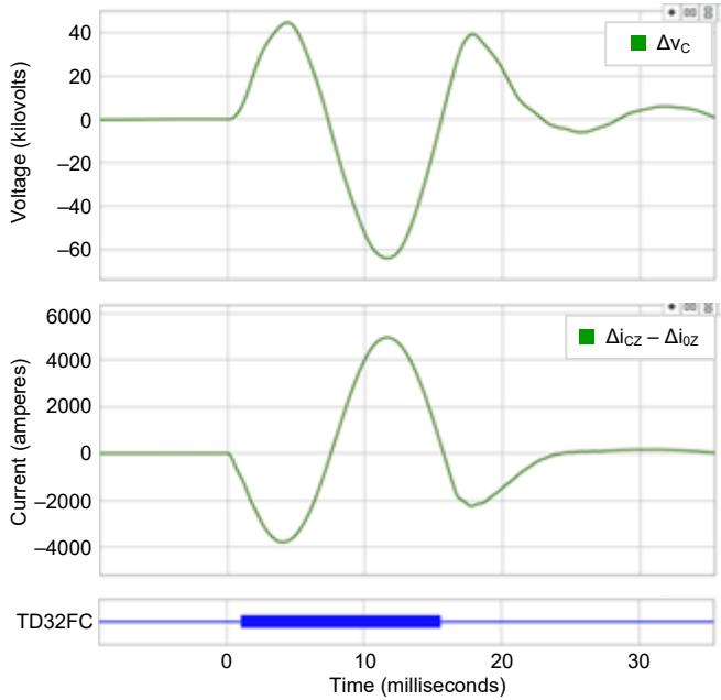
Fig. 30. Incremental voltage and replica current of the CG loop captured at MID and the TD32 protection element operation for the internal fault on May 4.
