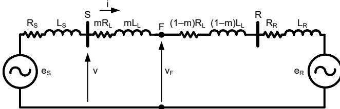
Fig. 2. Two-source single-phase system with a fault at F.
