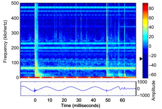
Fig. 22. Phase C (faulted phase) voltage waveform frequency content evolution over time.
