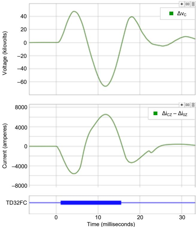
Fig. 31. Incremental voltage and replica current of the CG loop captured at TMD and the TD32 protection element operation for the internal fault on May 4.
