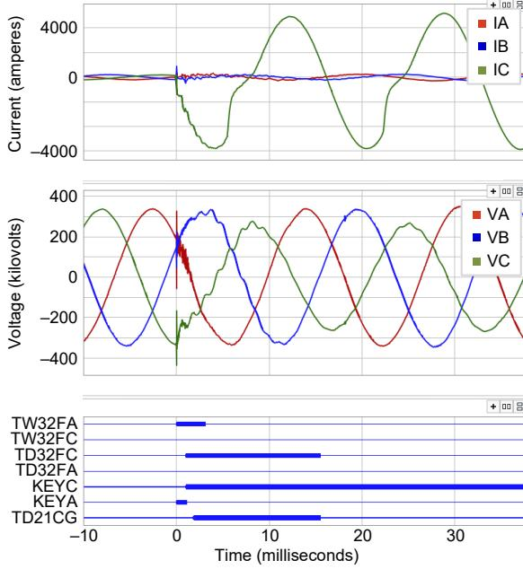
Fig. 27. Currents and voltages captured at TMD and the time-domain protection element operation for the internal fault on May 4.
