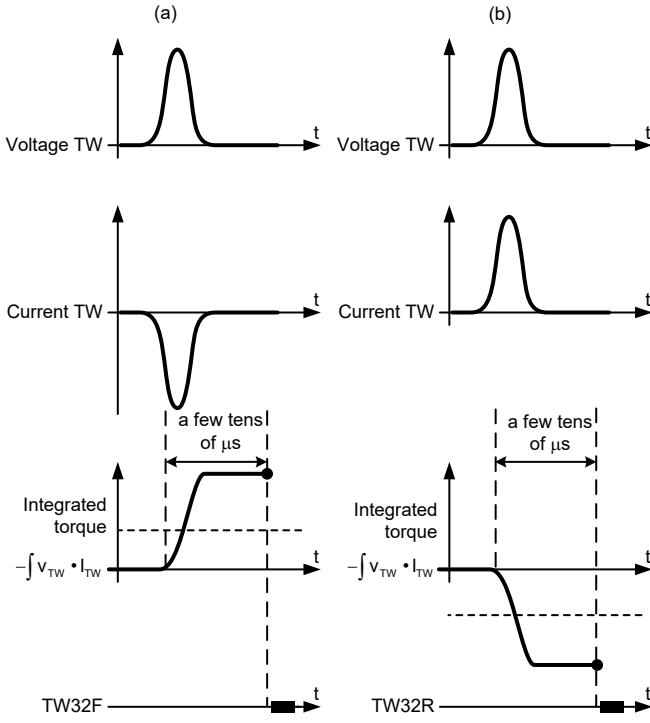
Fig. 9. Voltage and current TWs and the resulting integrated torques for (a) forward and (b) reverse faults.
