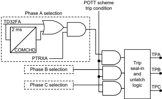
Fig. 18. Phase selection and trip logic for the POTT scheme.
