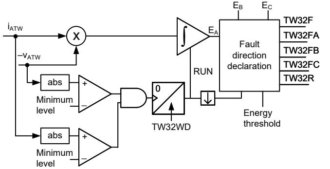
Fig. 8. Simplified logic of the TW32 element.
