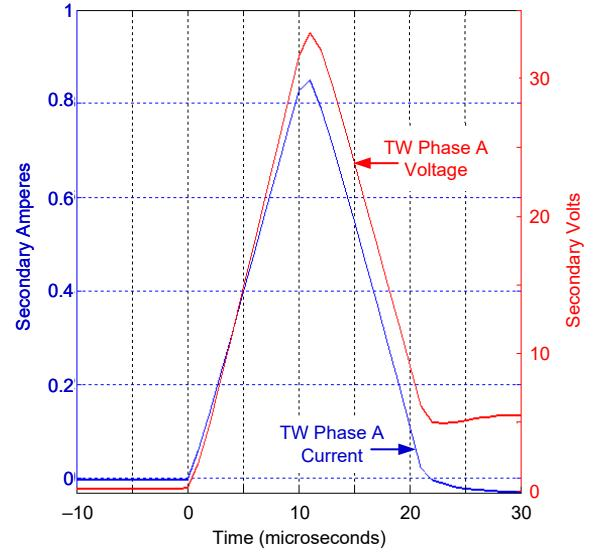
Fig. 13. The TW phase voltage and current of Circuit 2 at Terminal S have the same polarity for the fault shown in Fig. 11.
