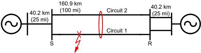
Fig. 11. An AG fault simulated on Circuit 1.
