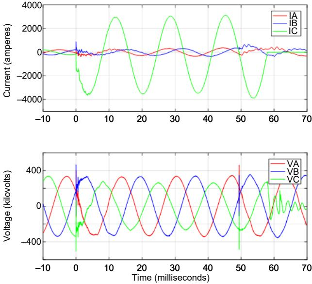
Fig. 19. Waveforms captured during a CG fault on a series-compensated 400 kV line.
