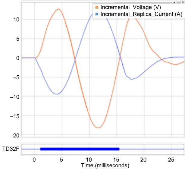
Fig. 6. The incremental voltage and incremental replica current have opposite polarities. Hence, the TD32 element declares the event as forward.
