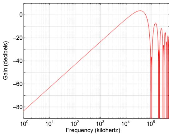
Fig. 23. Differentiator smoother filter frequency response.
