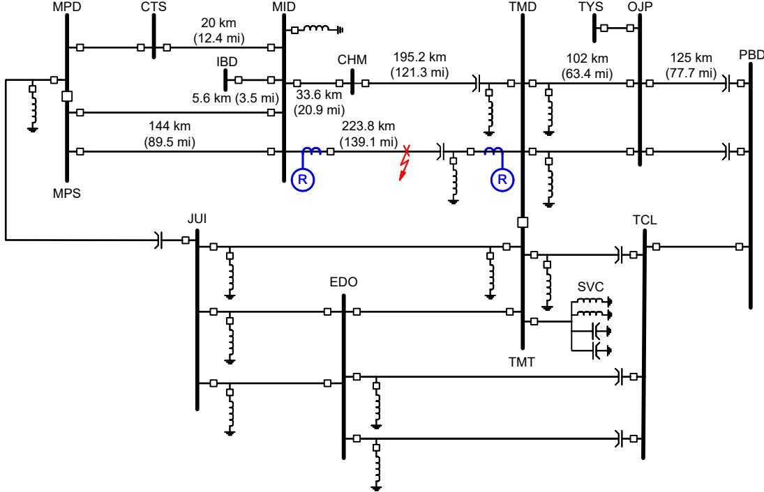
Fig. 25. Time-domain relays installed on the 400 kV line that connects the MID and TMD substations.
