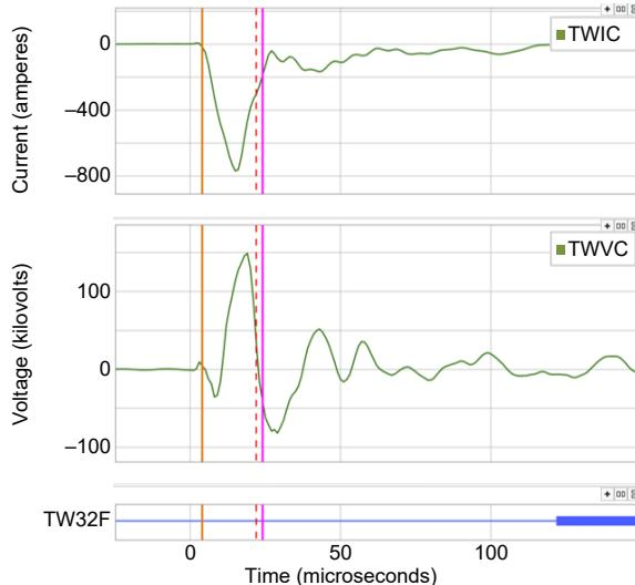
Fig. 24. TW phase current and voltage are of opposite polarities. Therefore, TW32 declared the event as forward.
