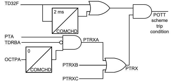
Fig. 17. Receiver logic provides security to the POTT scheme.
