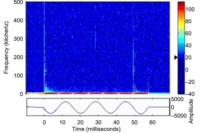
Fig. 21. Phase C (faulted phase) current waveform frequency content evolution over time.
