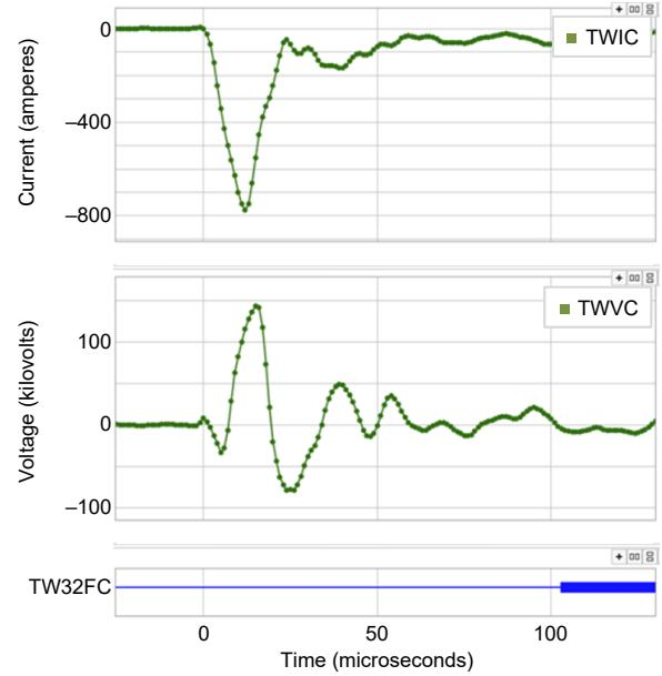
Fig. 28. TW current and voltage captured at MID and the TW32 protection element operation for the internal fault on May 4.
