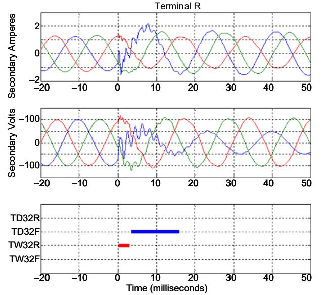
Fig. 14. The TW directional element declared the fault shown in Fig. 11 as reverse at Terminal R.
