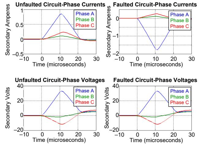
Fig. 10. Voltage and current TWs captured on a double-circuit line for an AG fault.
