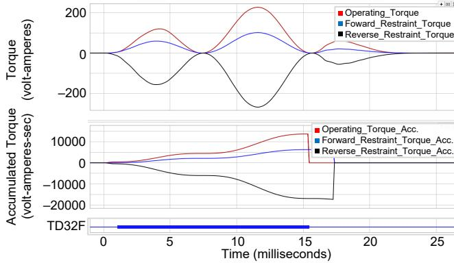
Fig. 7. The TD32 element declares the forward event when the accumulated operating torque is greater than the accumulated forward restraining torque.
