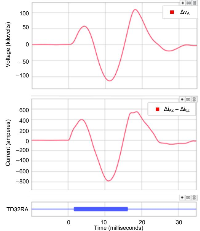
Fig. 33. Incremental voltage and replica current of the AG loop captured at MID and the TD32 protection element operation for the external fault on January 15.
