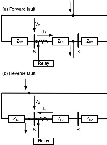
Fig. 1. Negative-sequence voltage and current for (a) forward and (b) reverse unbalanced faults.
