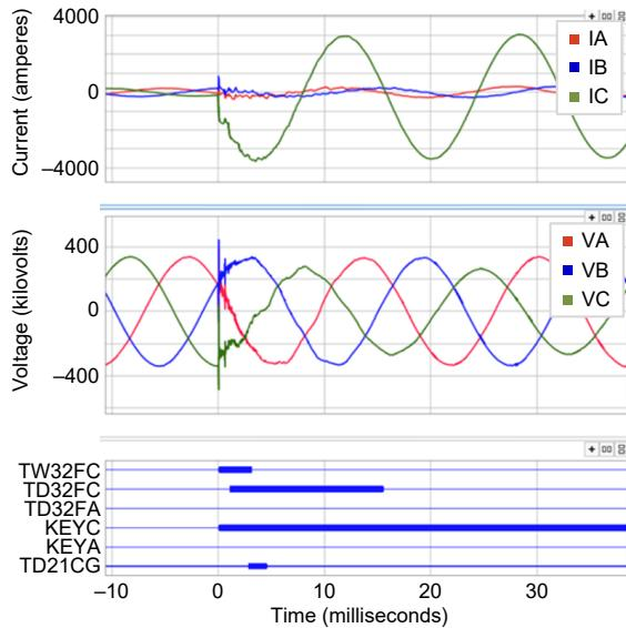
Fig. 26. Currents and voltages captured at MID and the time-domain protection element operation for the internal fault on May 4.
