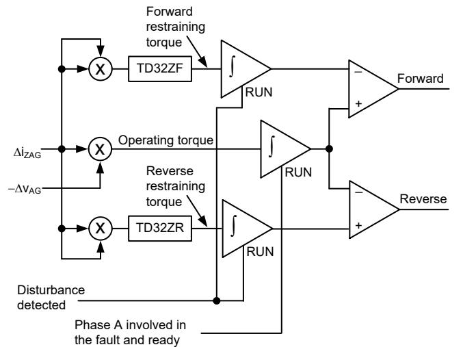
Fig. 5. Simplified logic of the TD32 element for the Phase-A-to-ground (AG) loop.
