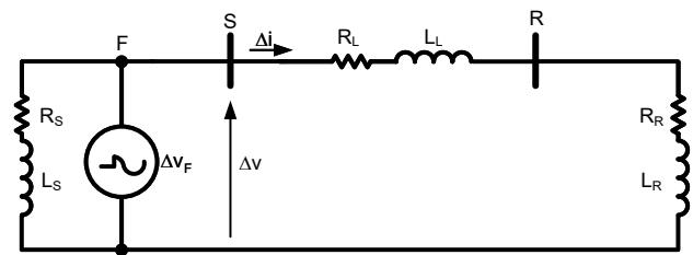
Fig. 4. Fault network of the Fig. 2 system for a fault behind Terminal S (a reverse fault for a relay at Terminal S).
