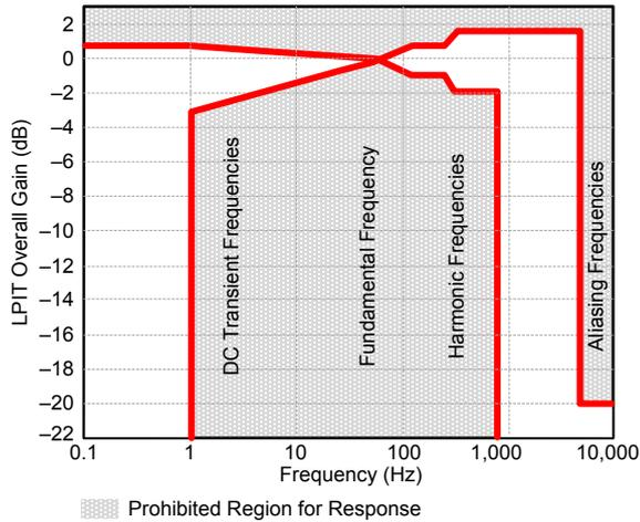
Fig. 6. Frequency response mask concept.
