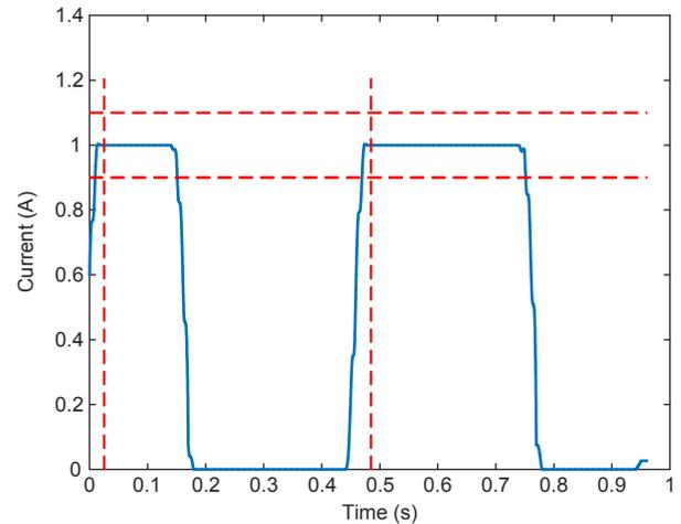
Fig. 9. Cycle-based rms value calculated for the SAMU output waveform in Fig. 7.
