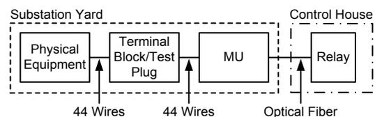
Fig. 2. Simplified diagram that shows cable reduction potential with Ethernet-based MU technology.
