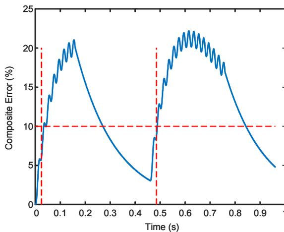
Fig. 8. Composite error calculated for the SAMU output waveform in Fig. 7.
