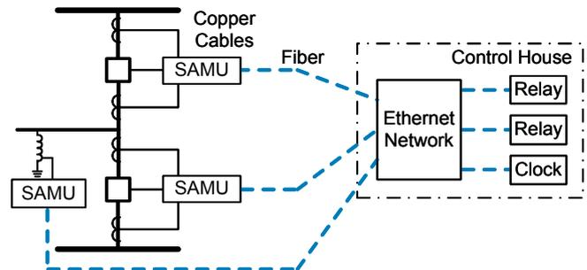
Fig. 3. Digital secondary system concept applied to an air-insulated HV substation.
