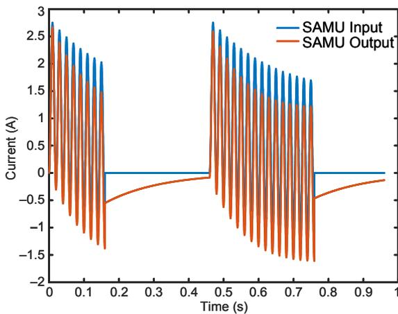
Fig. 7. Fully offset C-O-C-O sequence waveform before and after passing through a SAMU 1 Hz, high-pass filter.
