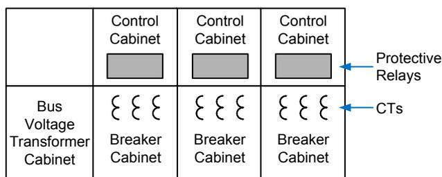
Fig. 4. Typical metal-enclosed MV switchgear.
