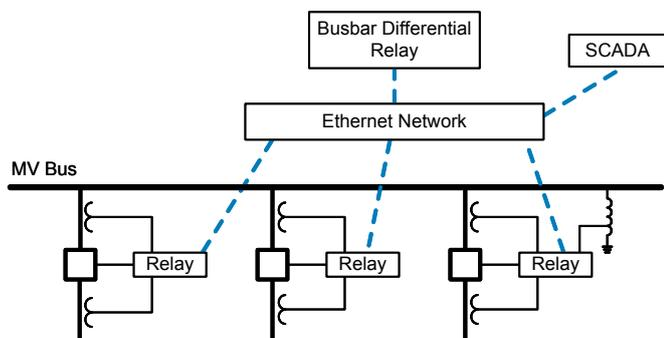
Fig. 5. Digital secondary system concept applied to metal-enclosed MV switchgear.
