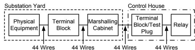
Fig. 1. Traditional wiring approach with relays in the control house.
