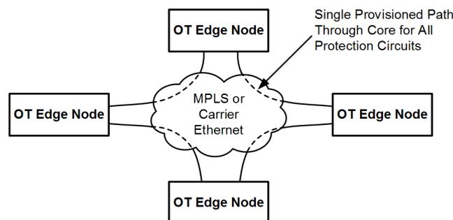
Figure 2 VSN Ring Topology Supported by Static Paths Through Core
