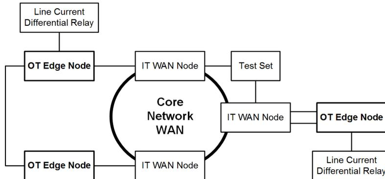
Figure 3 Performance Test Network Topology
