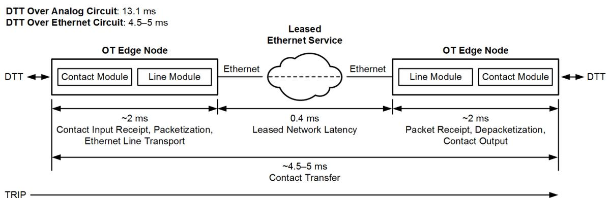
Figure 4 Live DTT Circuit Substation Results
