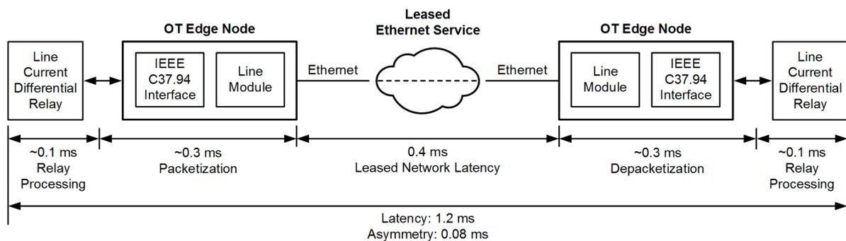
Figure 5 Live Line Current Differential Circuit Substation Results
