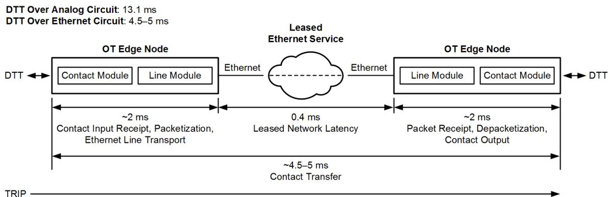
Figure 4 Live DTT Circuit Substation Results
