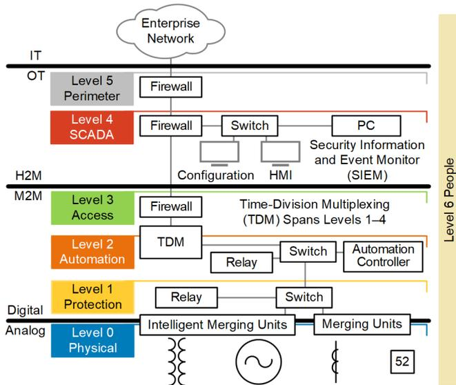
Fig. 1. ECS Defense-in-Depth Levels Diagram
