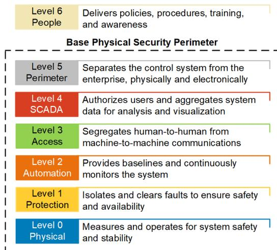
Fig. 2. Security Focus of Each Defense-in-Depth Level
