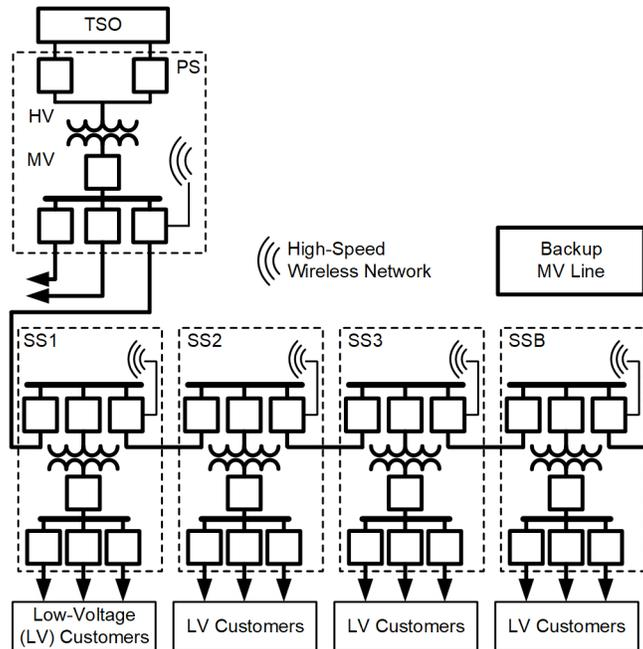
Fig. 1. Example portion of the E-Distribuzione electric network.
