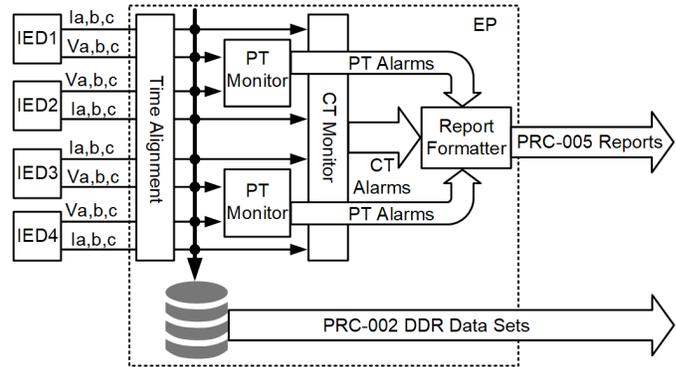
Fig. 3. Example PT/CT Monitoring System
