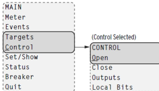
**Figure 4 Hidden information on a two-line display (dotted lines signify offscreen information).**
