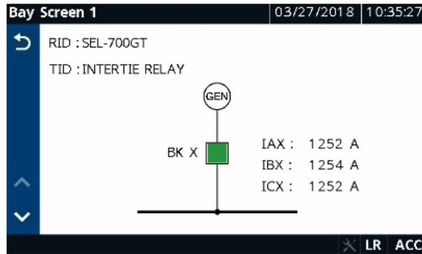
**Figure 3 SEL Bay Screen one-line diagram with real-time status indication.**
