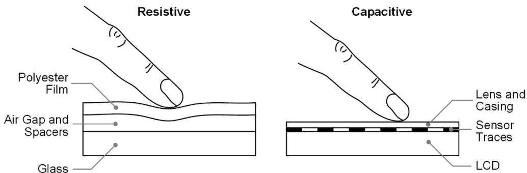
**Figure 1 Touchscreen internal structures.**
