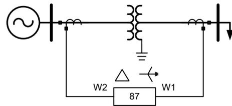
Fig. 12. Transformer current differential relay protecting a delta-wye transformer
