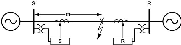
Fig. 9. Fault location on a two-source power system
