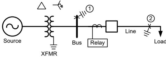
Fig. 6. Radial system with two fault locations
