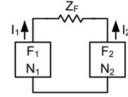
Fig. 4. Sequence network connections for a phase-to-phase fault
