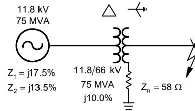
Fig. 7. One-line diagram for fault current calculations
